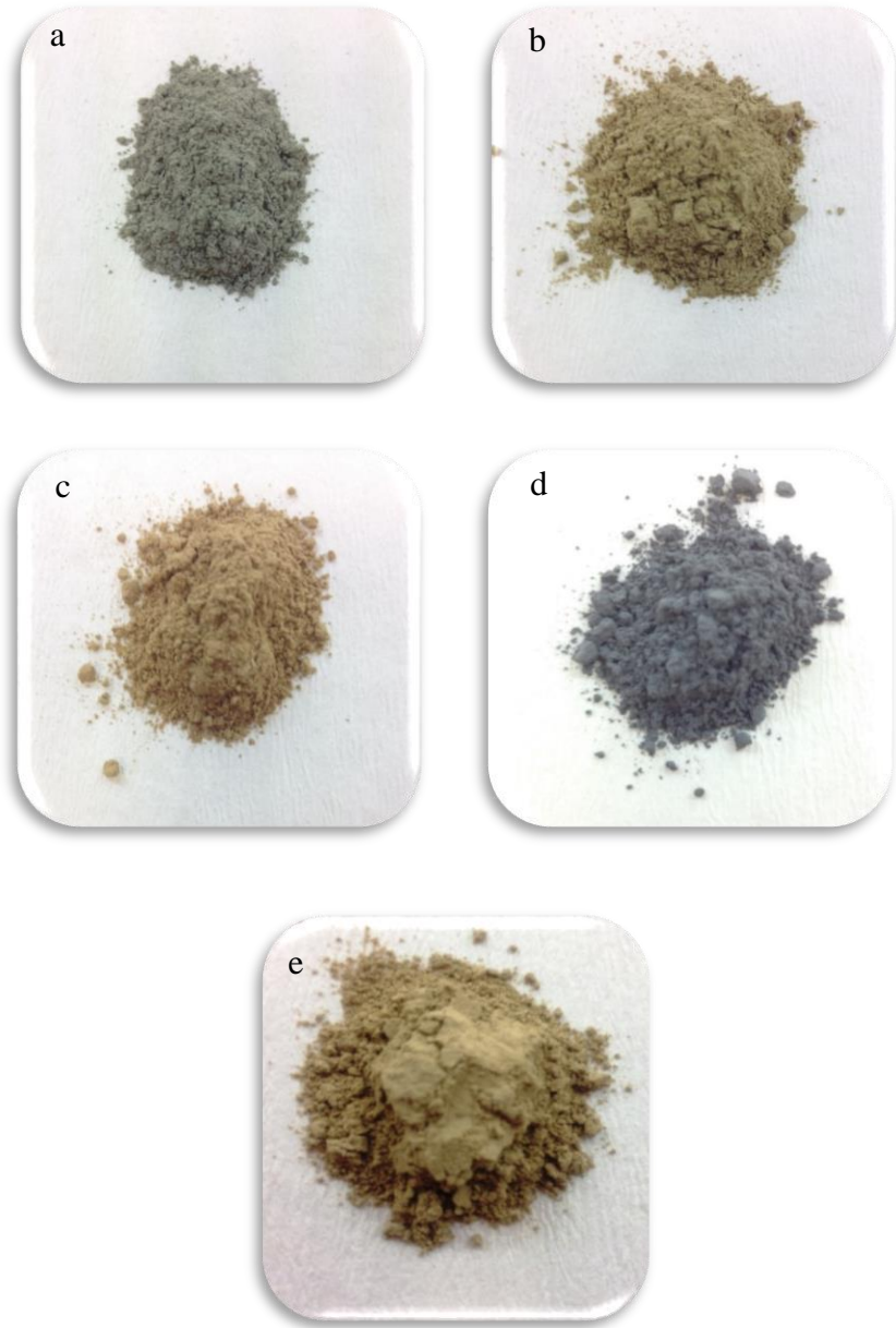
Figure 8. Ground powder schist-type samples ready for activation as a) G, b) C, c) P, d) B, and e) L
