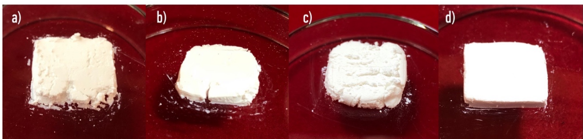
Figure 28 The wet cracking behavior of coagulated samples with a) AA100, b) AMPS100, c) VPA50, and d) the optimum additive, AMPS50
