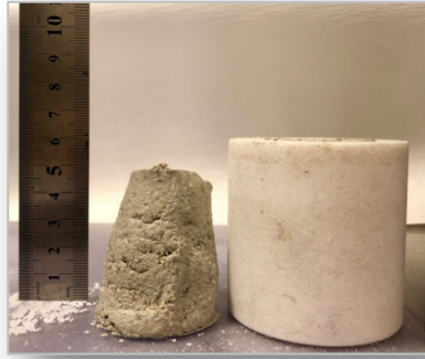
Figure 12 Mini slump test on FAC-20 mortar sample with 1 cm loss in height
