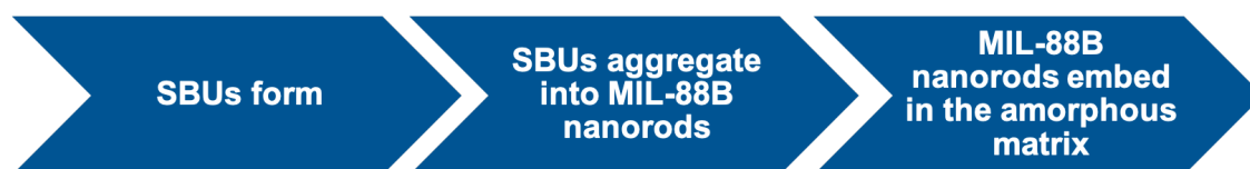
Figure 94. Schematic diagram of textural pore formation sequence.
