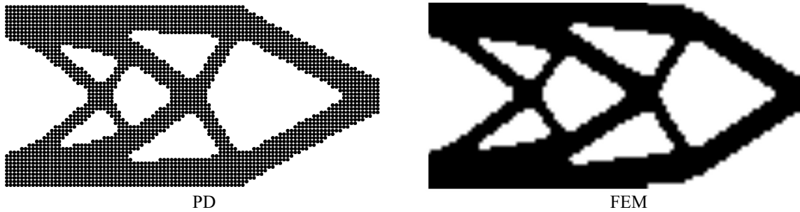
Figure 1. Comparison of design space discretization of FEM and PD for 100×50 particles in PD and elements in FEM.
