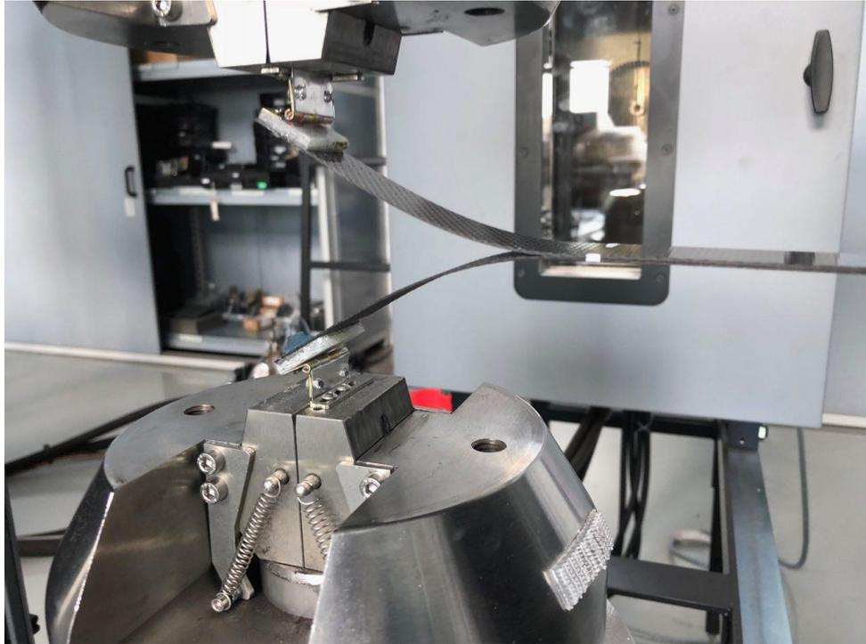
Figure 2.10 Mode-I fracture toughness test setup
