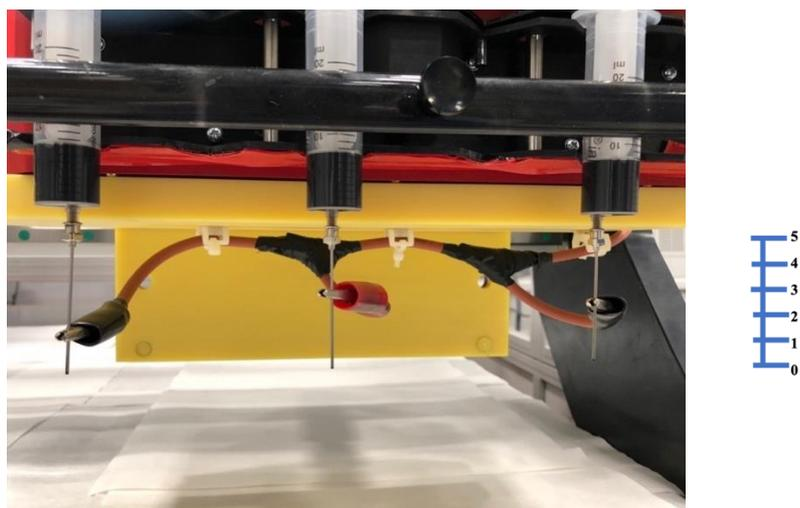
Figure 3.3 Positioning of crocodiles along syringe nozzles (Ideal positions #2,#4,#3)
