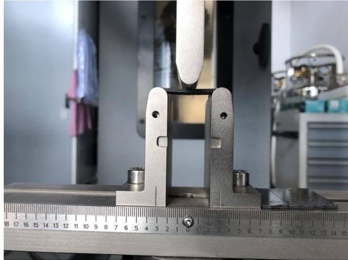
Figure 2.13 Three-point bending test setup
