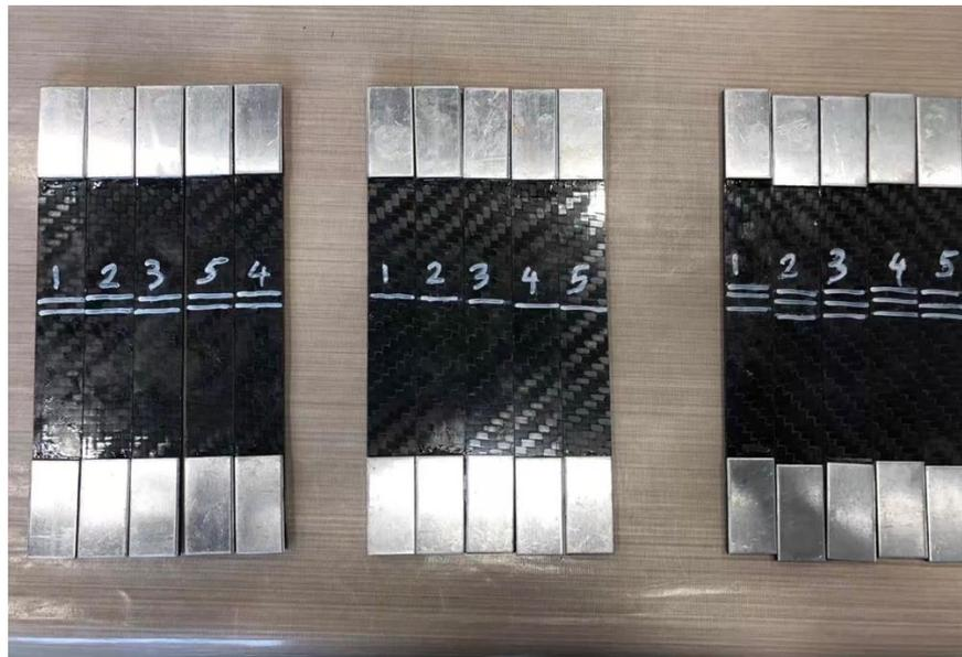
Figure 2.8 Tensile test specimens with aluminum tabs bonded on both ends
