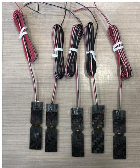
Figure 2.15 V-notched test specimens
