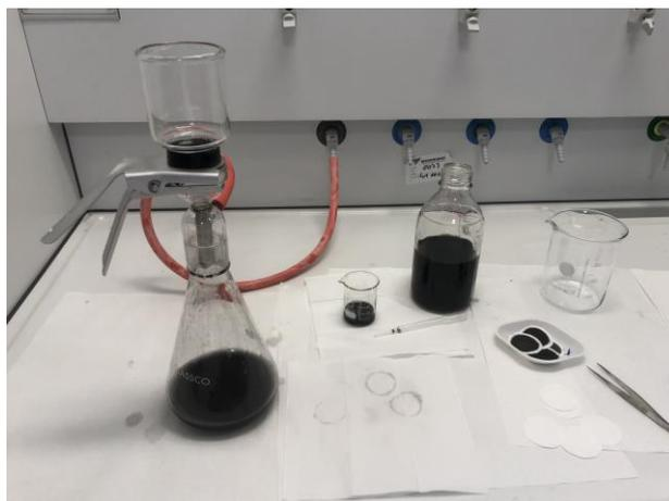
Figure 2.1 Vacuum filtration setup for SWCNT-H<sub>2</sub>O dispersions
