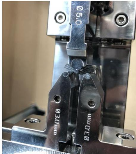
Figure 2.14 Short beam shear test setup
