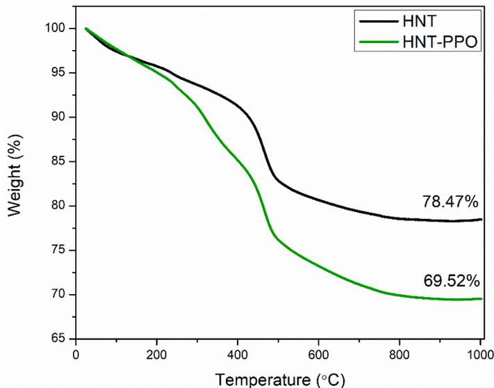
**Figure 30.** TGA curves for HNT and HNT-PPO under nitrogen atmosphere
