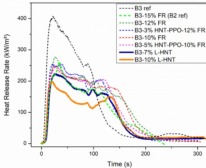
**Figure 43.** Heat release rate profiles of B3 foams incorporated with FR-loaded HNTs.
