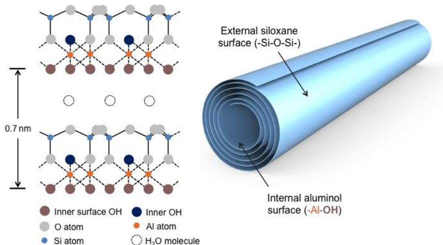
**Figure 2.** Halloysite nanotube [21]
