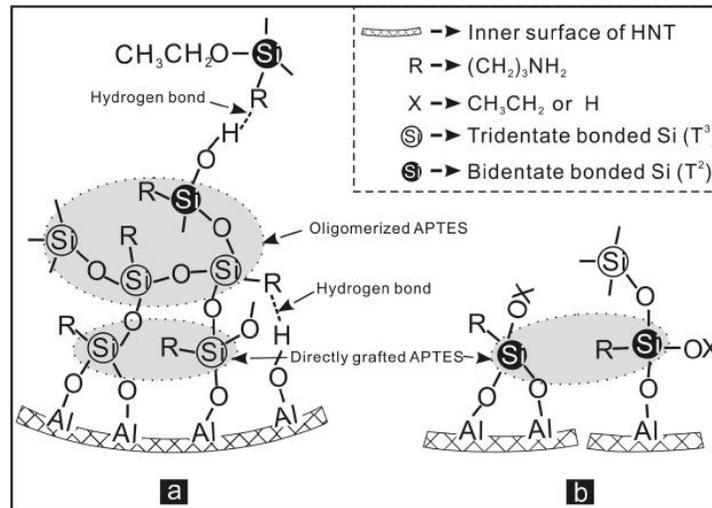
**Figure 4.** Formation of the crosslinked silane network [62]
