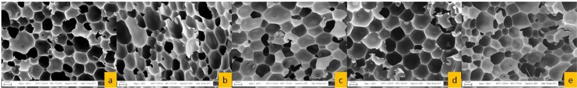
**Figure 17.** SEM images of DEC foams with sonicated HNT: (a) reference, (b) 1%, (c) 3%, (d) 5%, (e) 10%
