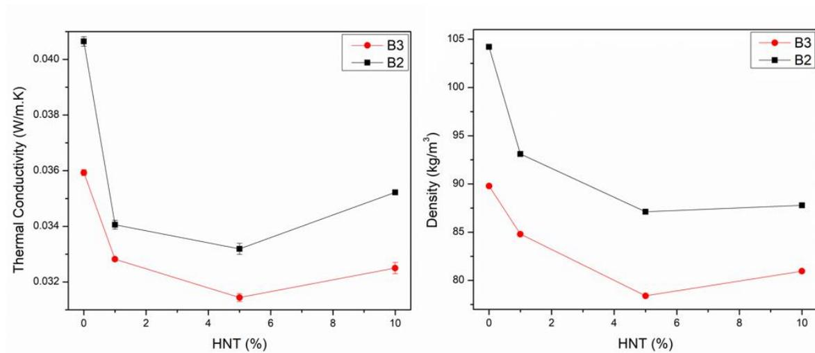
**Figure 24.** Thermal conductivity and density measurements for B3 and B2 foams
