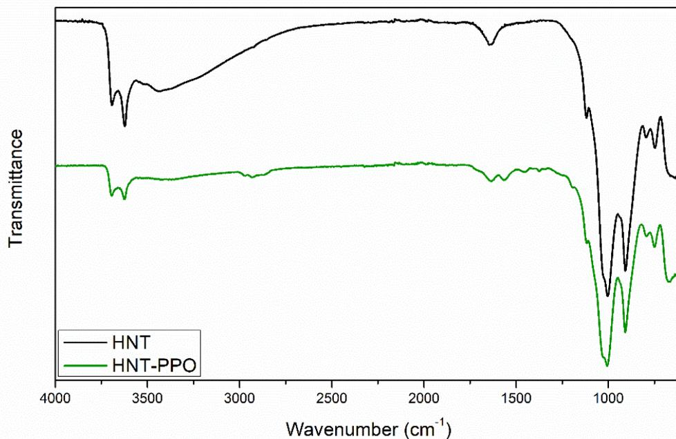
**Figure 29.** FT-IR spectra of reference HNT and HNT-PPO
