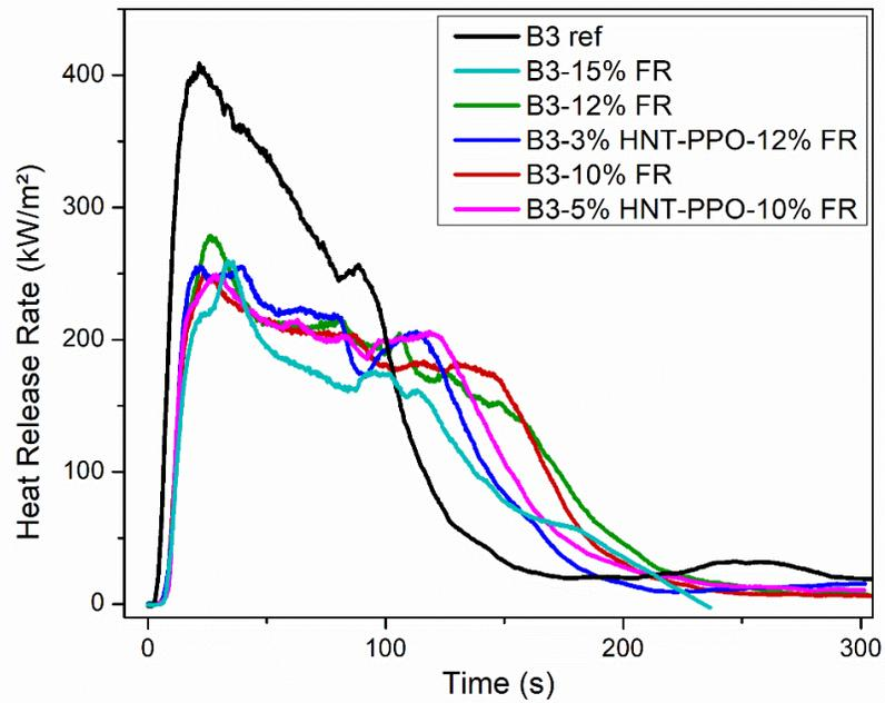
**Figure 41.** Heat release rate profiles of the samples
