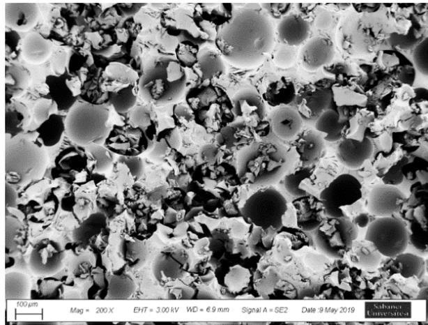
**Figure 15.** SEM image of foam resin after curing after unsuccessful evaporation of the blowing agent
