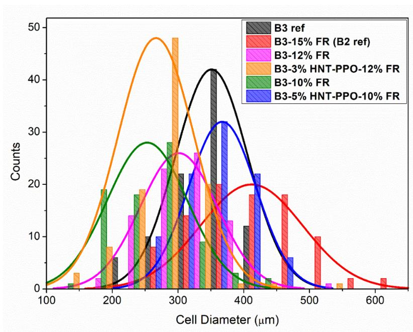
**Figure 32.** Cell size distribution of B3 foams prepared with HNT-PPO and FR
