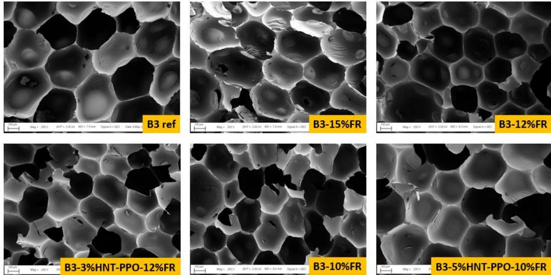
**Figure 31.** SEM images of B3 foams with HNT-PPO and FR
