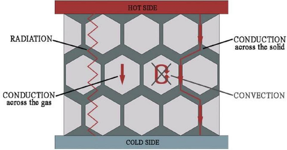
**Figure 11.** Heat transfer mechanisms in closed-cell polyurethane foams [92]
