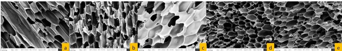
**Figure 19.** SEM images of SP foams with unprocessed HNT: (a) reference, (b) 1%, (c) 3%, (d) 5%, (e) 10%
