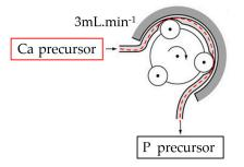
Reaction temperature: 45°C Ca/P: 1.55 Reaction pH: 5.5-8.0 Aging time: 24h Aging temperature: Room temperature Drying conditions: 80°C-overnight Sintering conditions: 600-900°C for 3h
