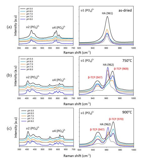
**Figure 7.** Raman spectra of the samples obtained at different conditions of pH and sintering temperature. The alterations in the  $(PO_4)^{3-} \nu 1$ ,  $\nu 2$ , and  $\nu 4$  vibration bands for each synthesis condition are given: (a) Corresponding vibration bands of the as-dried samples; (b) corresponding vibration bands of the samples sintered at 750 °C; (c) corresponding vibration bands of the samples sintered at 900 °C.
