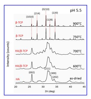
**Figure 2.** XRD patterns of the samples that were synthesized at pH 5.5. The effect of the sintering temperature on the chemical transformation of Ca-deficient hydroxyapatite (CDHA) to  $\beta$ -tricalcium phosphate ( $\beta$ -TCP) is revealed. Transformation to  $\beta$ -TCP is almost complete as early as 750 °C.
