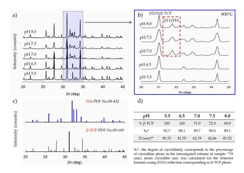
**Figure 4.** XRD investigation of the samples that were sintered at 900 °C: (**a**) For the range of  $20-45^{\circ}$ ; (**b**) for the range of  $30-35^{\circ}$ ; (**c**) XRD spectra of standard HA (No:09-0432) and  $\beta$ -TCP (No: 09-0169); (**d**) calculated percentage of transformed  $\beta$ -TCP, average crystallite size, and the degree of crystallinity. The transformation from CDHA to  $\beta$ -TCP was completed for the samples that were synthesized under pH 5.5 and pH 6.5.
