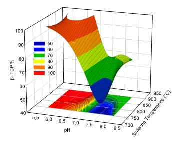
**Figure 5.** The percentage of transformation depending on the reaction pH and sintering temperature. Among all the synthesis and sintering conditions, a complete transformation of CDHA to  $\beta$ -TCP was only observed for the pH 5.5/750 °C and pH 5.5–6.5/900 °C samples.
