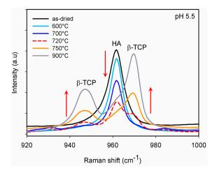
**Figure 6.** Raman spectra of the samples that were synthesized at pH 5.5. The effect of sintering temperature on the chemical transformation of CDHA to  $\beta$ -TCP is revealed by tracking the most characteristic v1 mode. Transformation to  $\beta$ -TCP is started at 720 °C and is almost complete as early as 750 °C.
