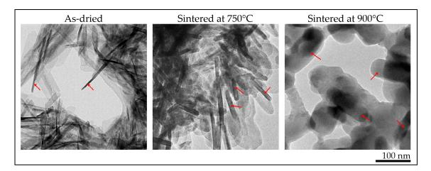
**Figure 8.** Bright-field TEM micrographs of the as-dried and sintered samples, which were synthesized at pH 5.5. After sintering at 750 °C, pure  $\beta$ -TCP is obtained, keeping its initial as-dried morphology with slightly thicker needle-like structures.
