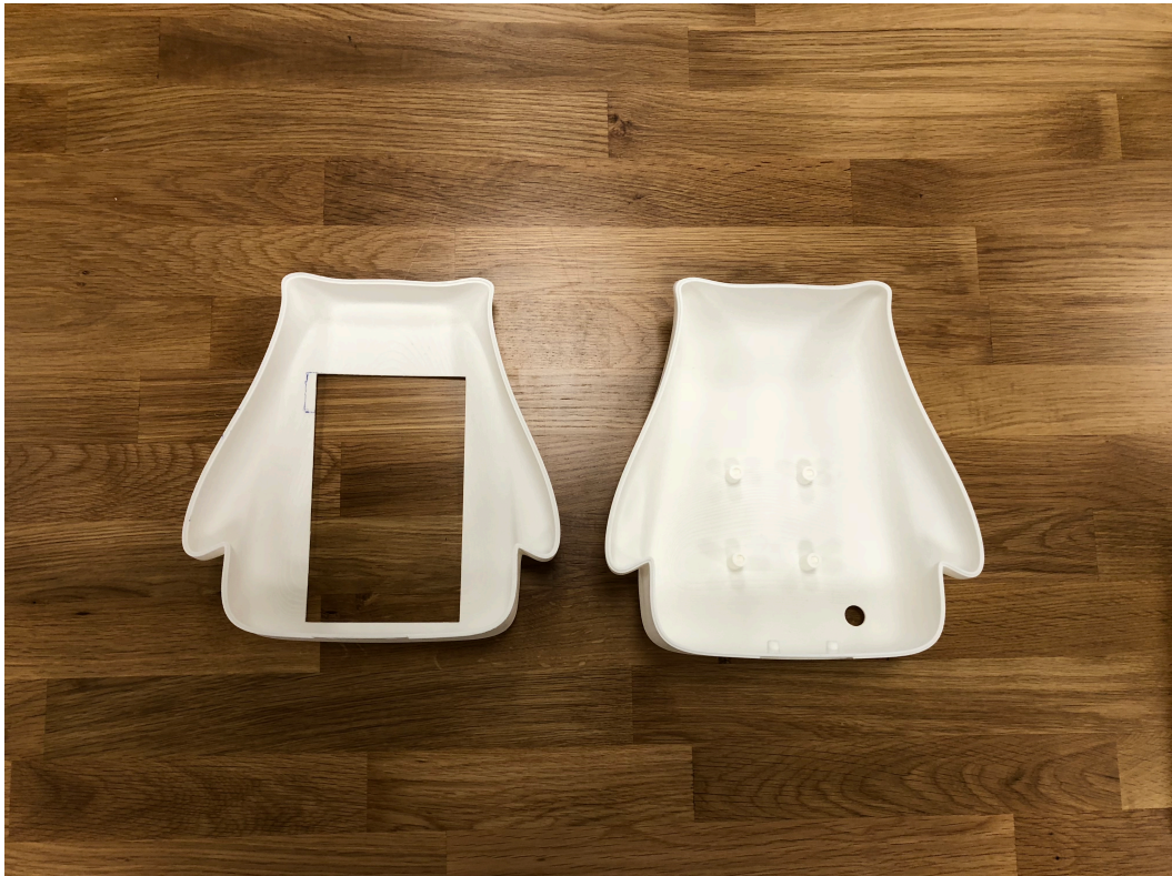
Figure 35. 3D printed shell components, back
