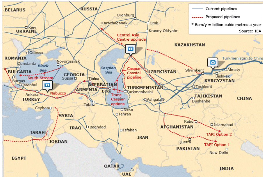
Figure 8: Gas Pipelines to China
