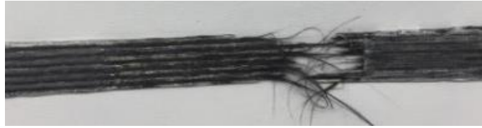
Figure 55: Without tabbed trial sample's observed fracture.
