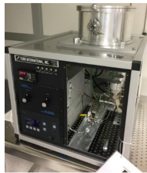
Figure 30: Torr International Inc. machine, used for oxygen plasma.
