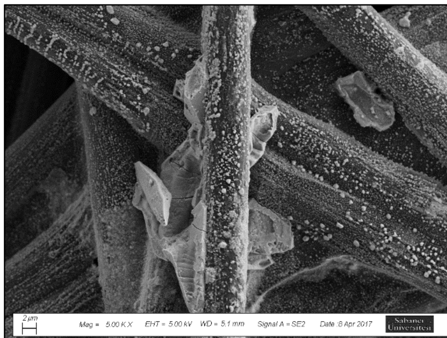
Figure 11. SEM micrograph of Pt/GO/CP electrophoretically deposited at 10 V/240 minutes.
