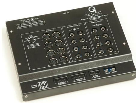
FIGURE 4.7: Quanser Q8 Data Acquisition Card.
