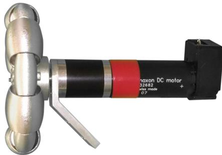
FIGURE 4.4: Omniwheel-actuator connection.
