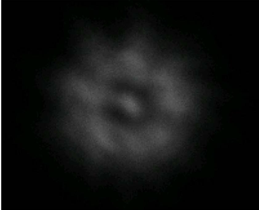
Figure 6-20: Image of the fiber mode acquired by the camera, used to perfectly align the two interferometer arms.
