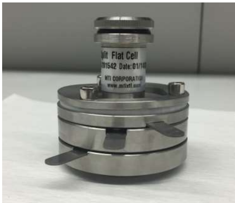
Figure 22. Assembled lithium-ion battery
