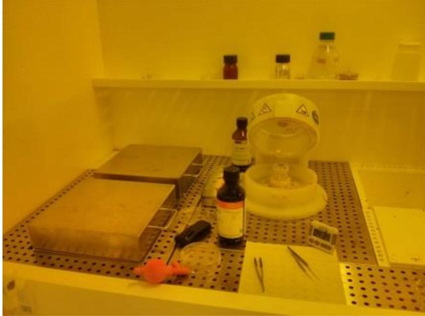
**Figure 29:** Spin coating equipment and materials for laying resist in yellow-room
