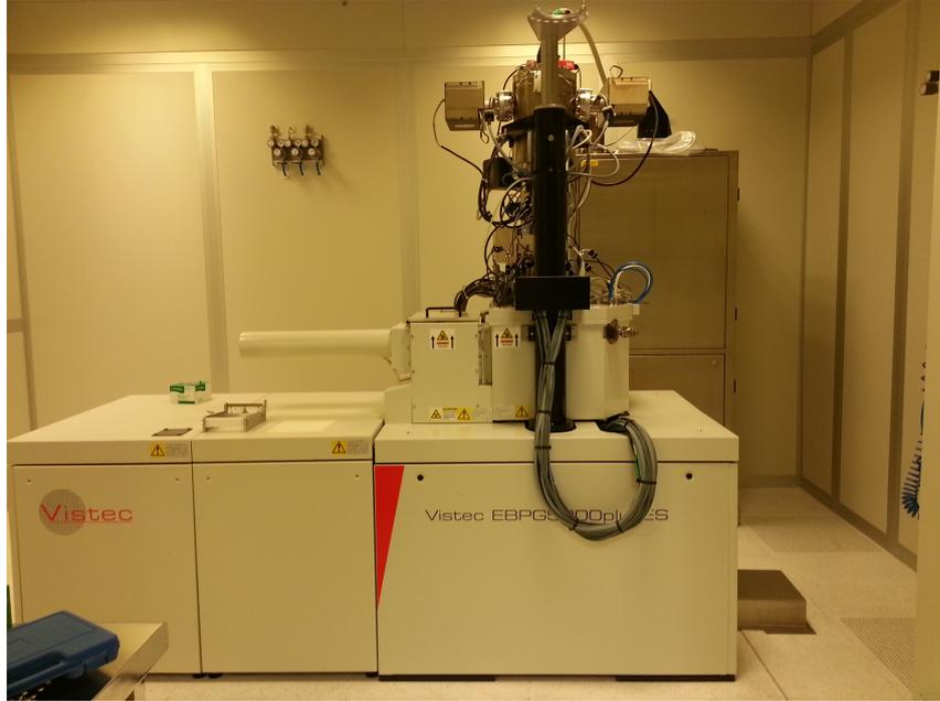
**Figure 28:** Electron beam lithography (EBL) system in Sabanci Univeristy SUNUM cleanroom facilities
