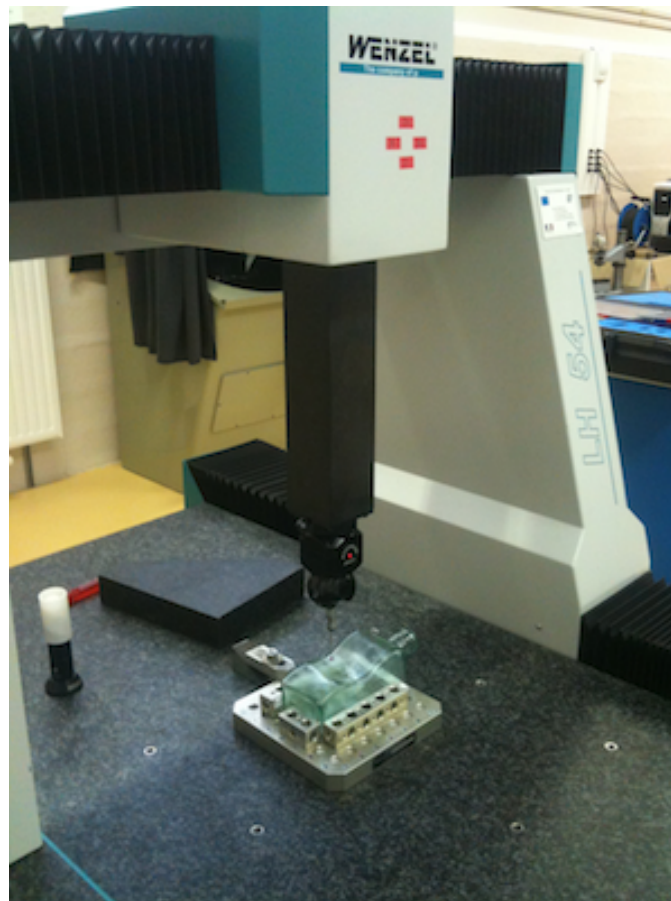
Figure 5.28: Scanning of the glass bottle by Wenzel LH 54 touch probe scanner.
