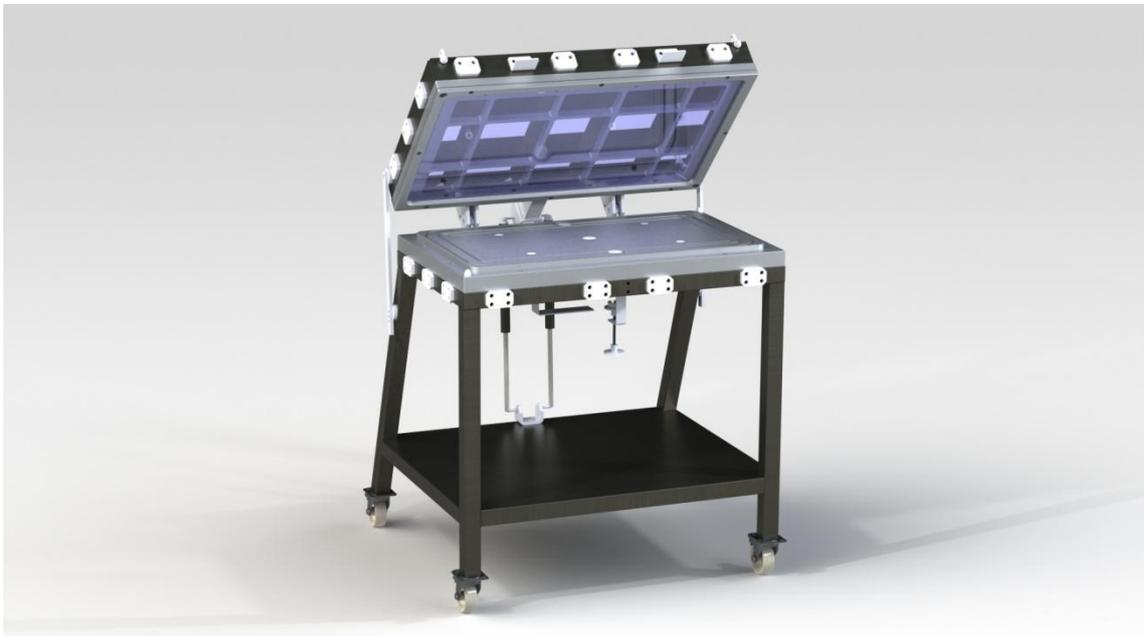
**Figure 3.3: Render image of the new RTM**
