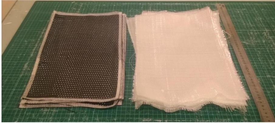
**Figure 4.5: Reinforcements**
