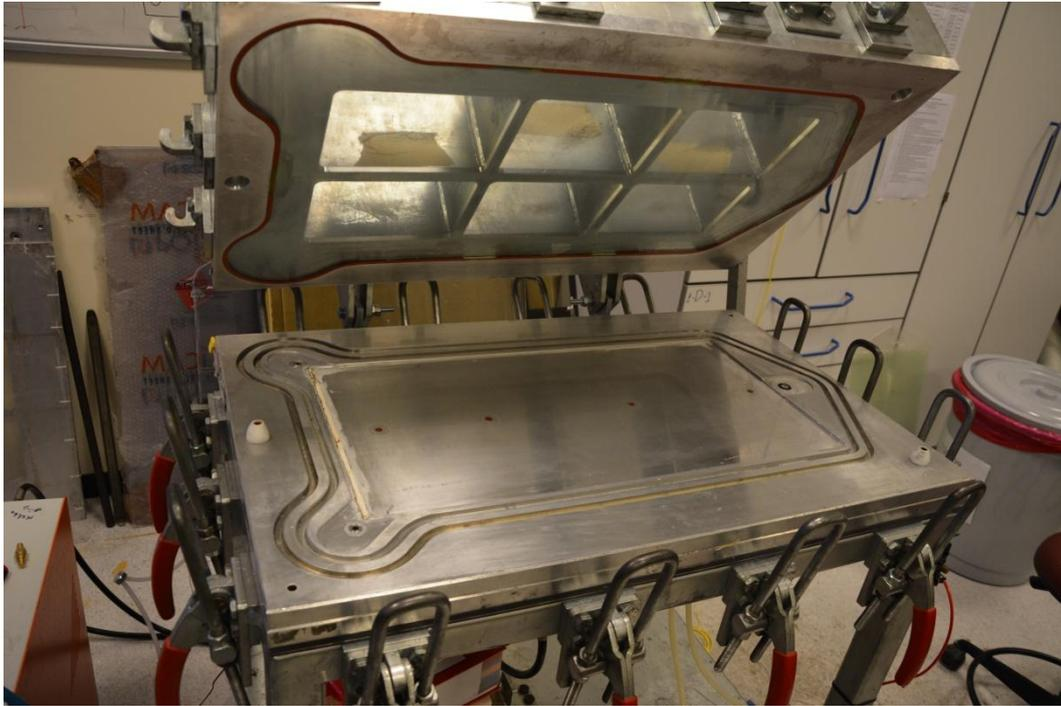
**Figure 3.2: Revised RTM; shape of the glass is similar to o-ring path**
