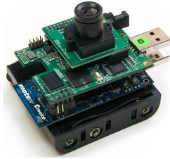
**Figure 2.7:** The nodes in VSNs consist of image sensor, embedded processor and wireless transceiver.
