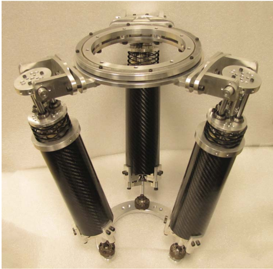
Figure 3.11: First prototype of ASSISTON-ANKLE and its series elastic actuator.
