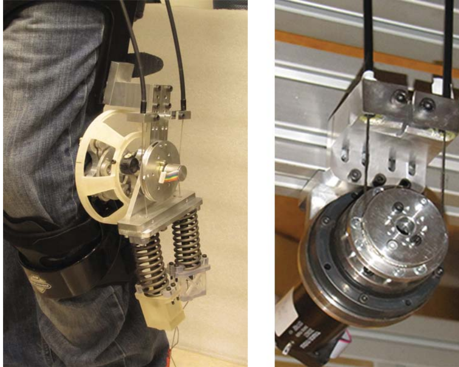
Figure 2.8: ASSISTON-KNEE and its remote actuation unit
