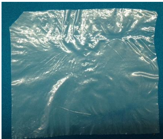
Figure C.1: ETFE- g -4VP high temperature proton conducting membrane. Radiation dose: 10 kGy, grafting solvent: n -propanol, GL: 42%
