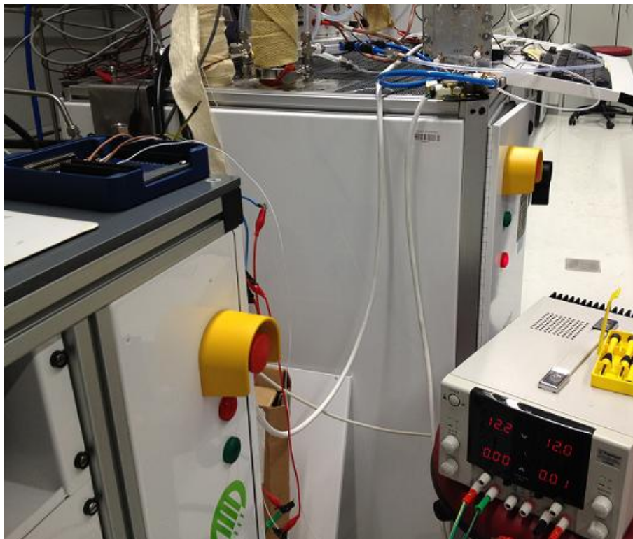
Figure B.2: Connecting the solenoid valves to the NI 6220 Digital Output
