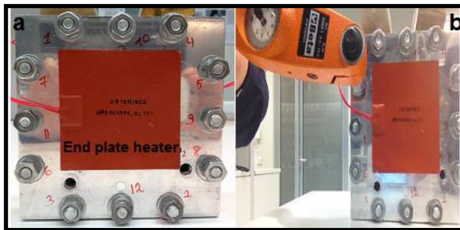
Figure 4.6: The applied torque to assemble the test cell
