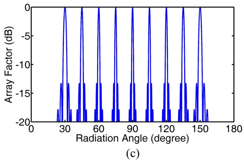
**Figure 5:** Normalized array pattern of a linear array with  $\lambda/2$  spacing for (a)  $N=8$  (b)  $N=32$  (c)  $N=100$  antenna elements
