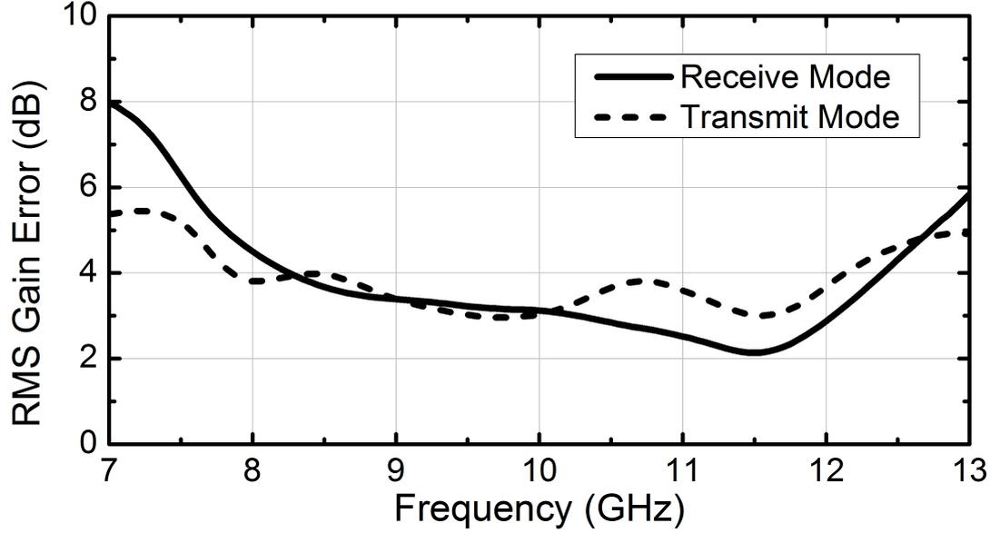
**Figure 67:** Measured RMS gain error of T/R module in receiver and transmitter modes
