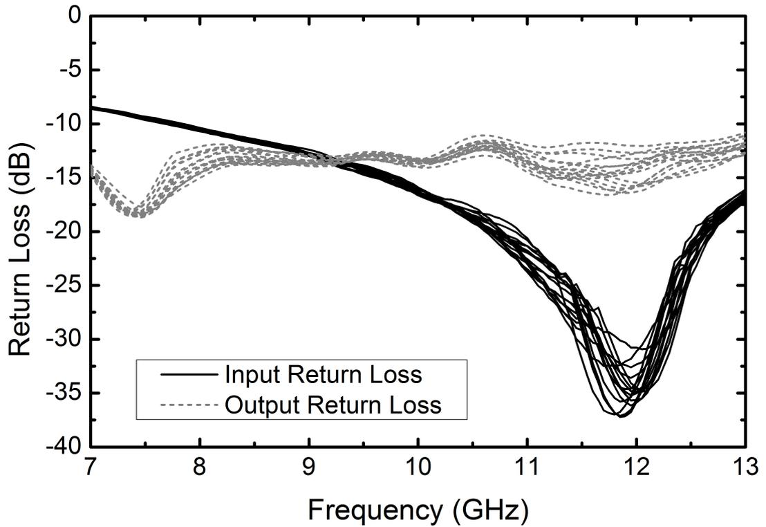
**Figure 57:** Measured input and output return losses of T/R module in receiver mode for all phase states
