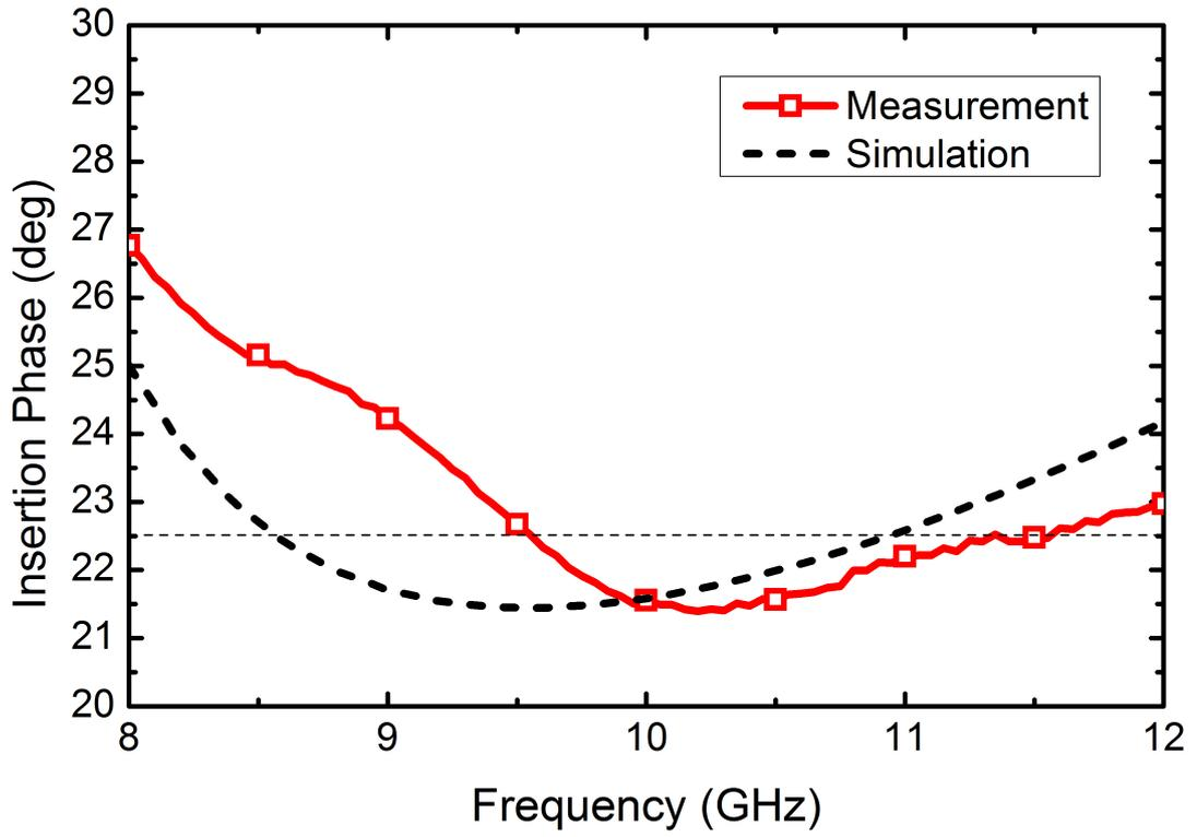
**Figure 35:** Simulated and measured phase shift of 22.5° bit.
