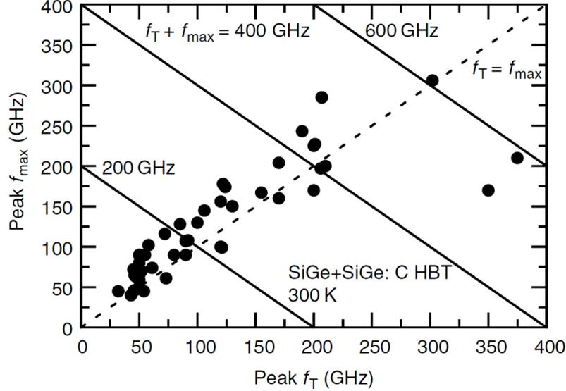
**Figure 10:** Cutoff frequency ( $f_T$ ) and maximum oscillation frequency ( $f_{MAX}$ ) for different SiGe HBT technologies. [2]
