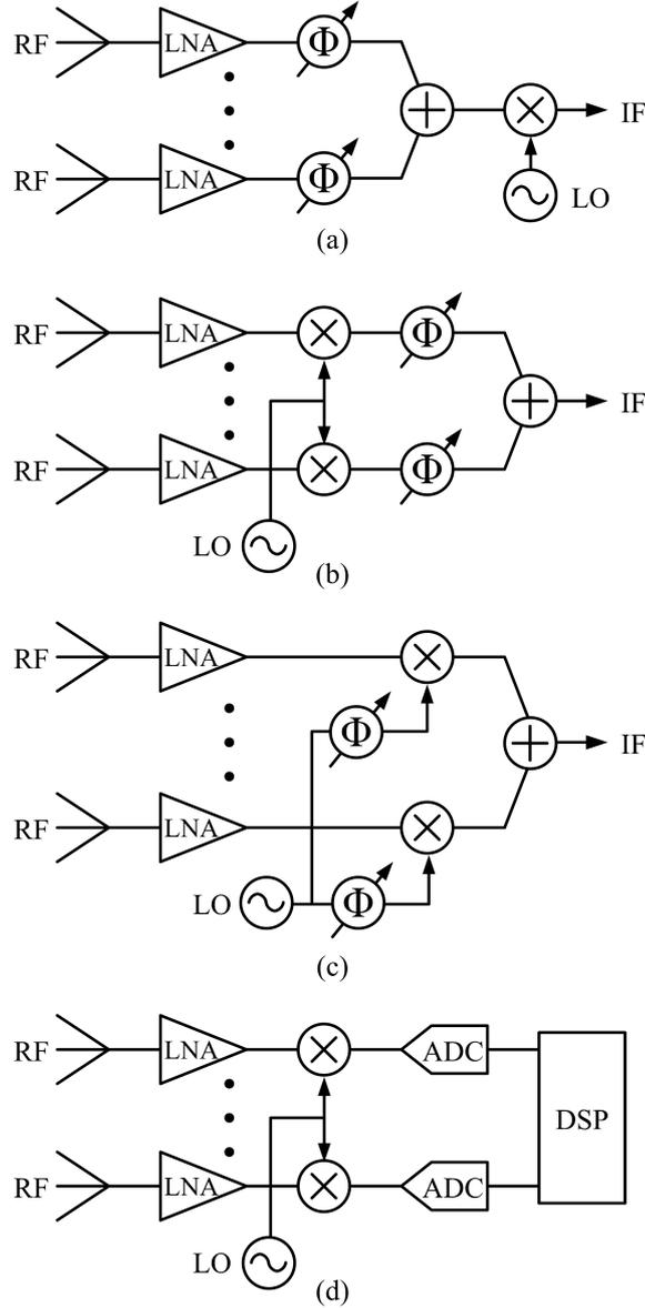
**Figure 7:** Phased array architectures: (a) RF phase shifting (b) IF phase shifting (c) LO phase shifting (d) Digital beam forming
