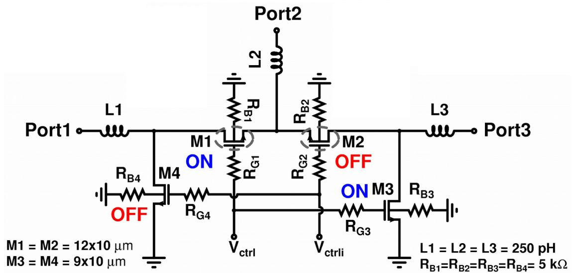
Figure 42: Schematic view of the SPDT switch
