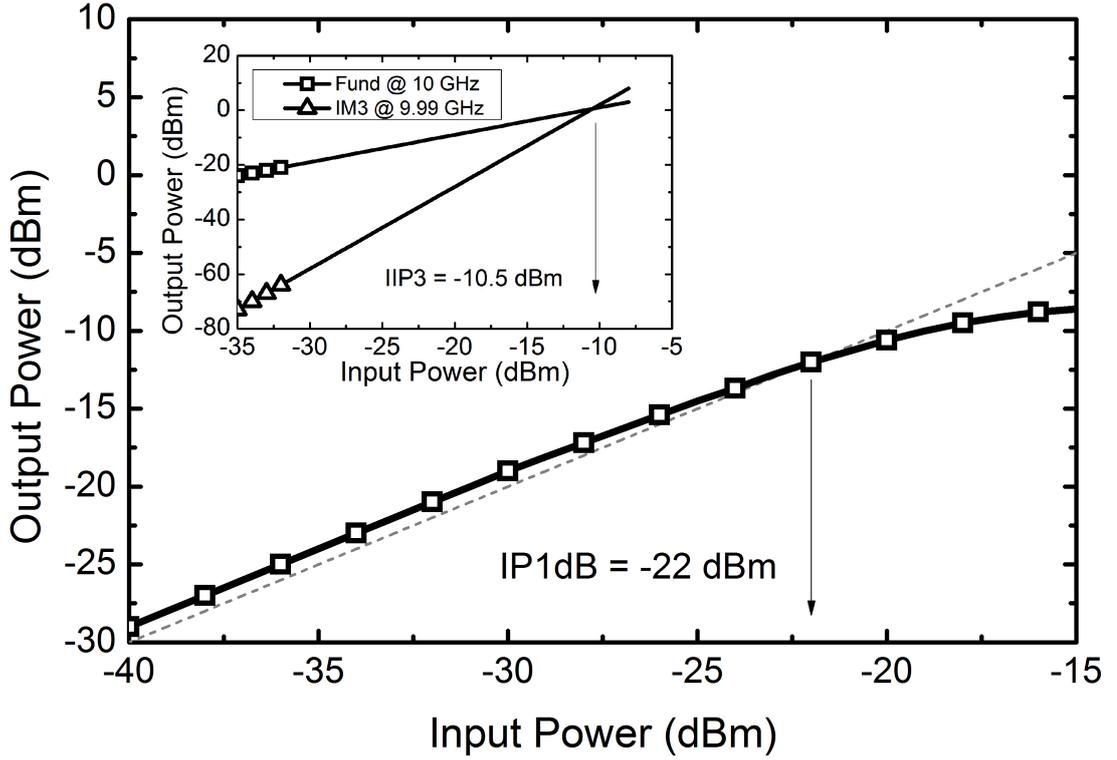
**Figure 63:** Measured 1-dB compression point and third order intercept point of T/R module in receiver mode
