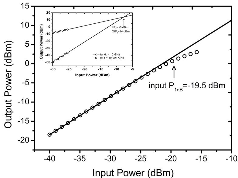
**Figure 49:** Single-tone and two-tone linearity measurement results of the LNA.
