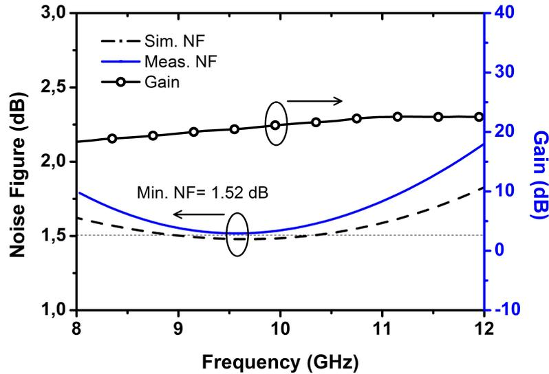
**Figure 48:** Gain and noise figure of the LNA.
