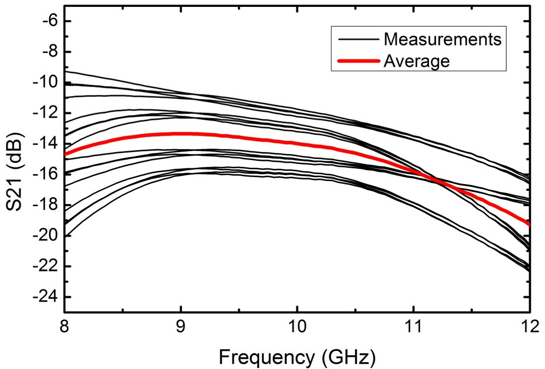
**Figure 34:** Extrapolated insertion losses of the 4-bit phase shifter from the measurements of standalone phase shifter bits.
