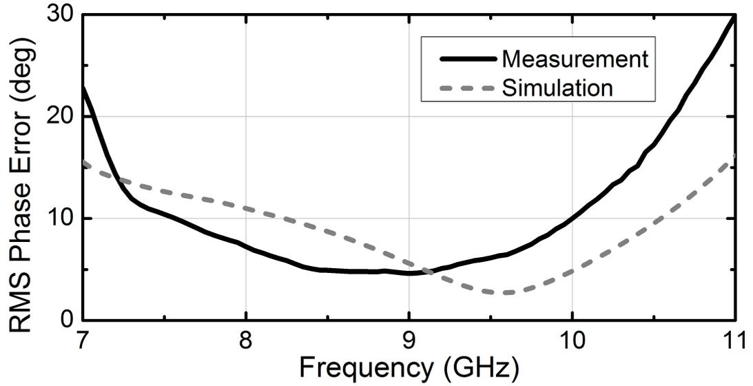
**Figure 62:** Simulated and measured RMS phase error T/R module in receiver mode
