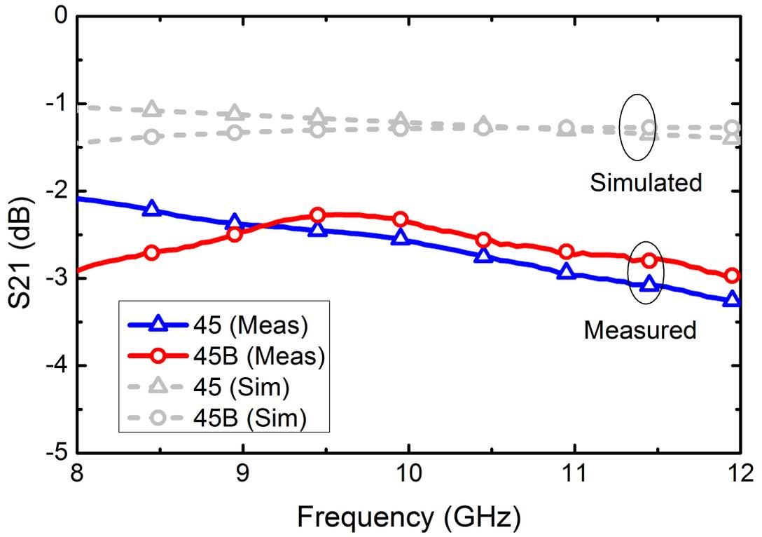
**Figure 31:** Simulated and measured insertion losses of  $45^\circ$  bit in both phase shift and bypass modes.
