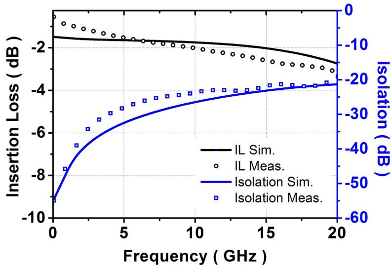
**Figure 44:** Simulated and measured insertion loss and isolation of the SPDT switch
