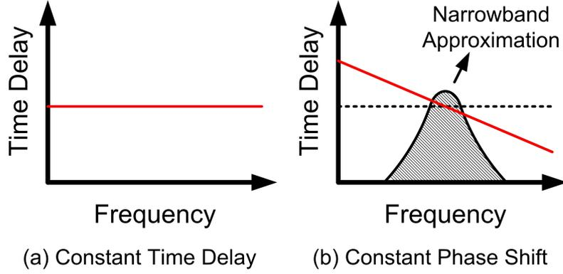
**Figure 4:** Narrowband phase shift approximation for time delay
