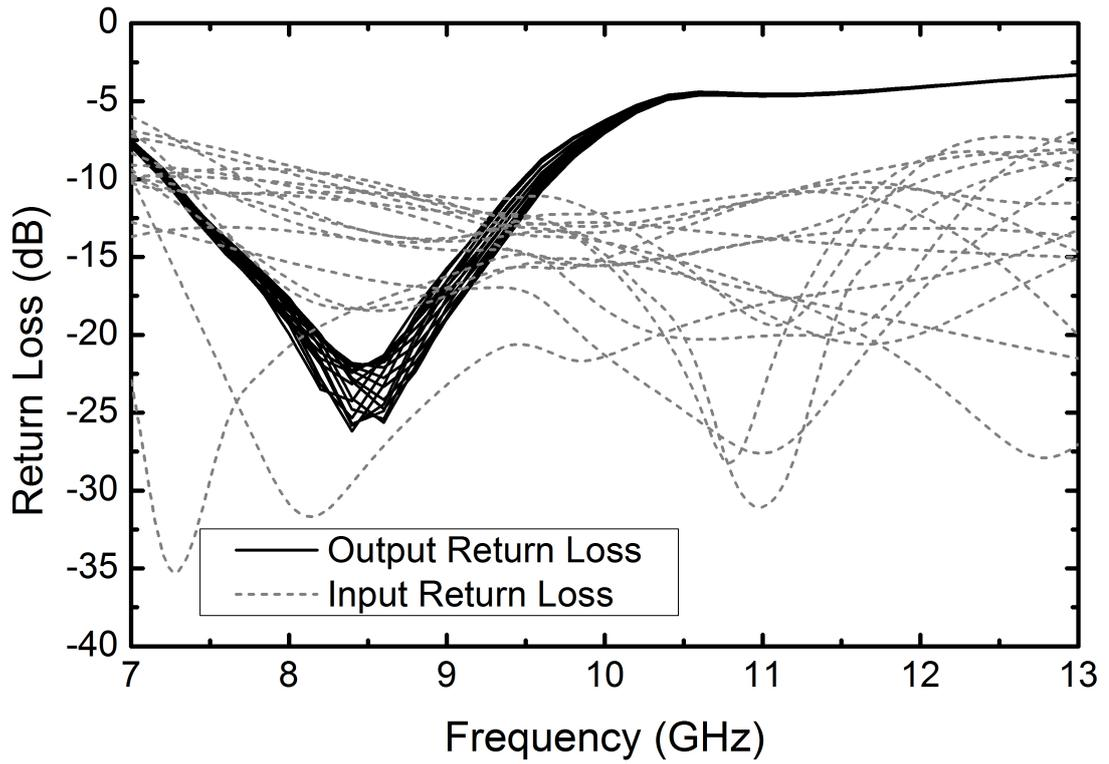
**Figure 64:** Measured input and output return losses of T/R module in transmitter mode for all phase states
