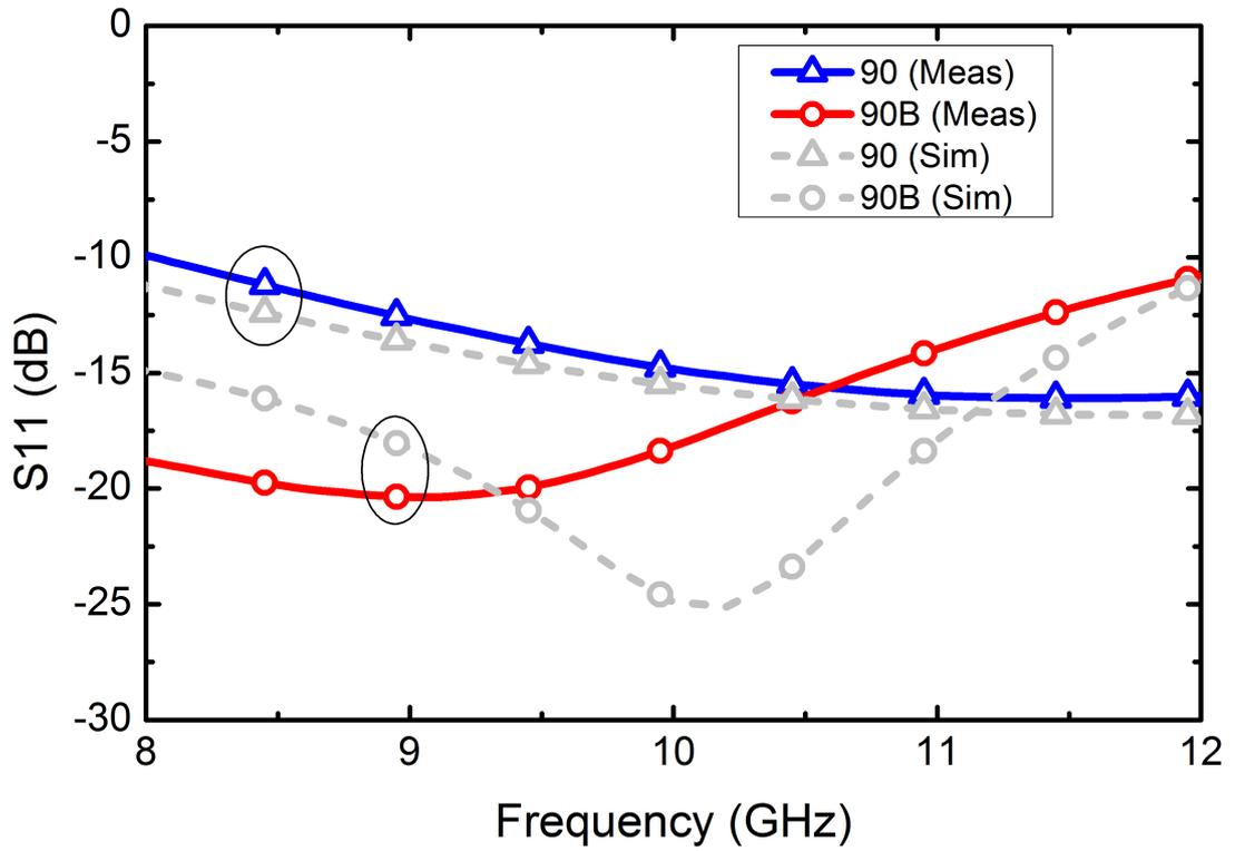
**Figure 28:** Simulated and measured return losses of  $90^\circ$  bit in both phase shift and bypass modes.
