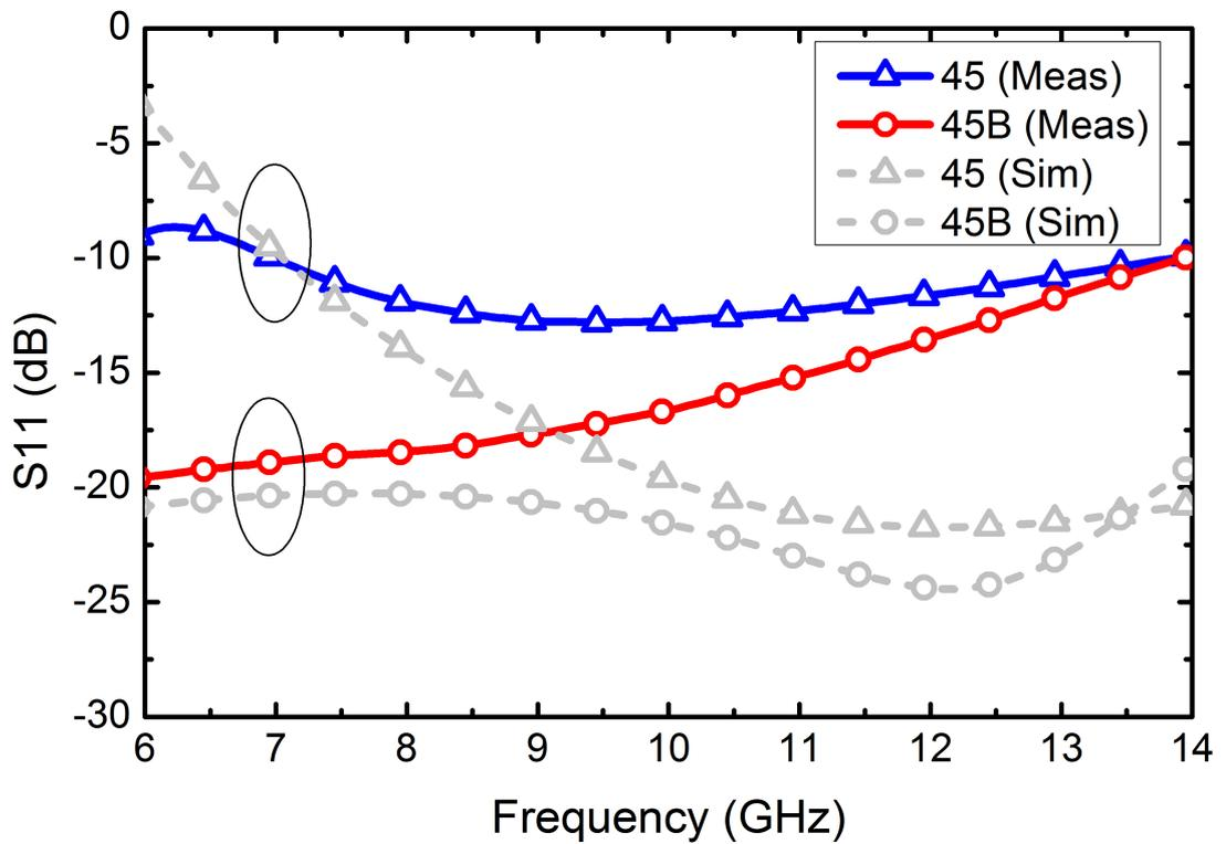
**Figure 27:** Simulated and measured return losses of 45° bit in both phase shift and bypass modes.
