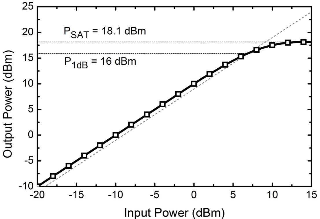
**Figure 66:** Measured 1-dB compression point and saturated output power of T/R module in transmitter mode
