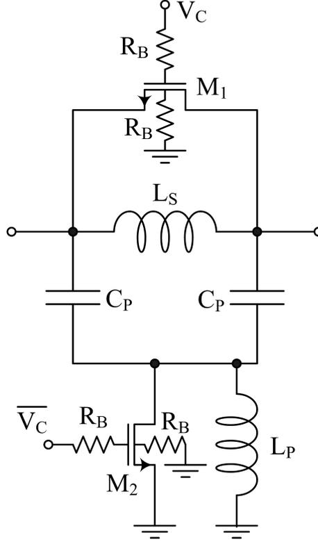
**Figure 22:** Switched filter phase shifter topology
