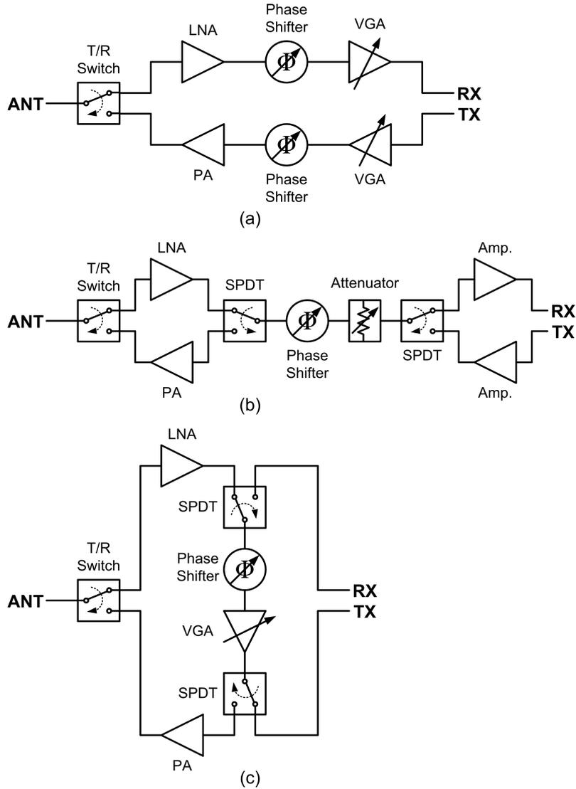
**Figure 8:** Several system level architectures for RF transmit/receive modules
