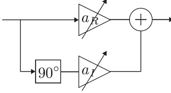
**Figure 17:** Vector modulator phase shifter [4]
