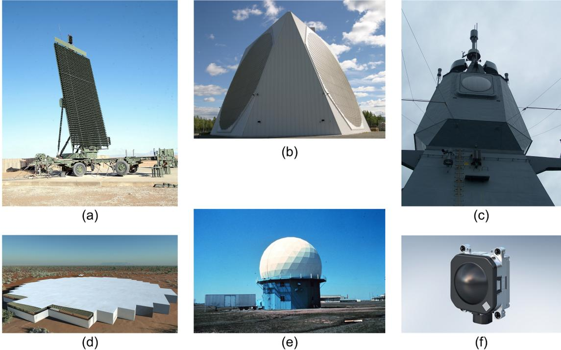
**Figure 1:** Various military (a-c) and commercial (d-f) phased array radars
