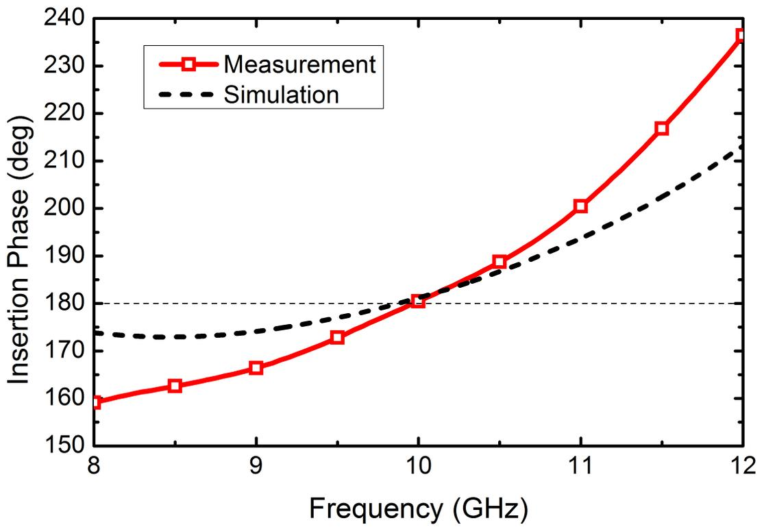
Figure 38: Simulated and measured phase shift of 180° bit.
