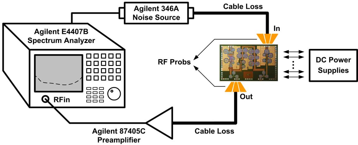
Figure 59: Noise figure measurement setup
