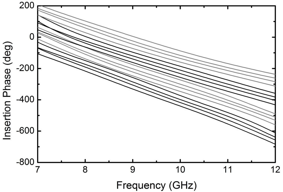
**Figure 61:** Measured insertion phase of T/R module in receiver mode for all phase states
