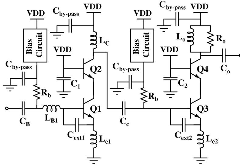
Figure 46: Schematic view of the two stage LNA.
