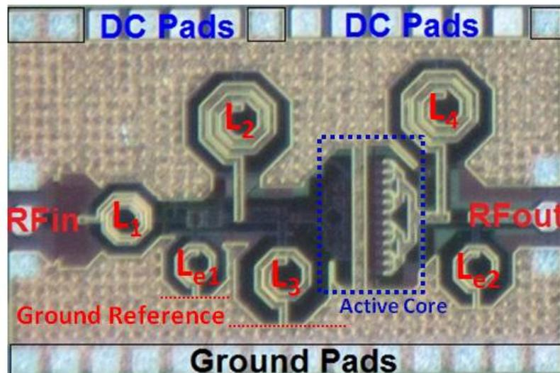
Figure 51: Chip photo of the fabricated PA.
