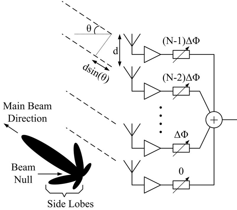
**Figure 3:** Basic phased-array receiver block diagram.
