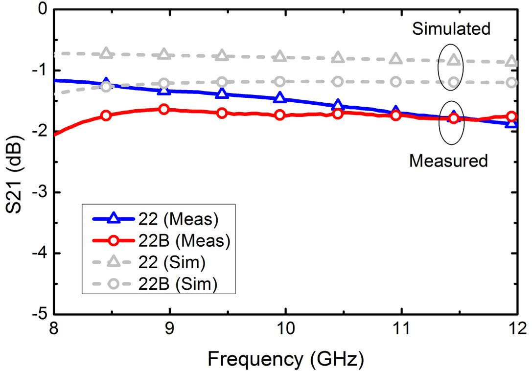
**Figure 30:** Simulated and measured insertion losses of  $22.5^\circ$  bit in both phase shift and bypass modes.
