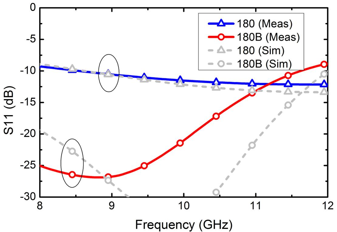
**Figure 29:** Simulated and measured return losses of  $180^\circ$  bit in both phase shift and bypass modes.
