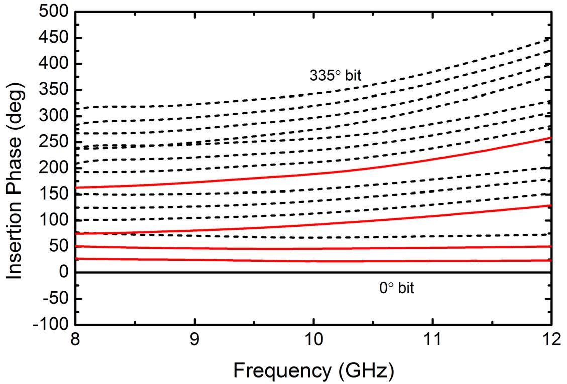
Figure 39: Extrapolated 16 phase states from the measurements of 4 standalone phase shifter bits.
