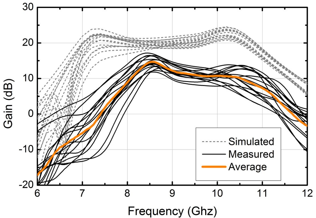
**Figure 65:** Simulated and measured gain T/R module in transmitter mode for all phase states
