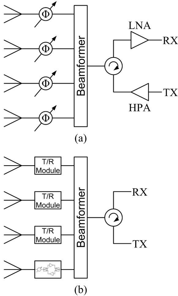
**Figure 6:** Block diagram of (a) passive phased arrays and (b) active phased arrays
