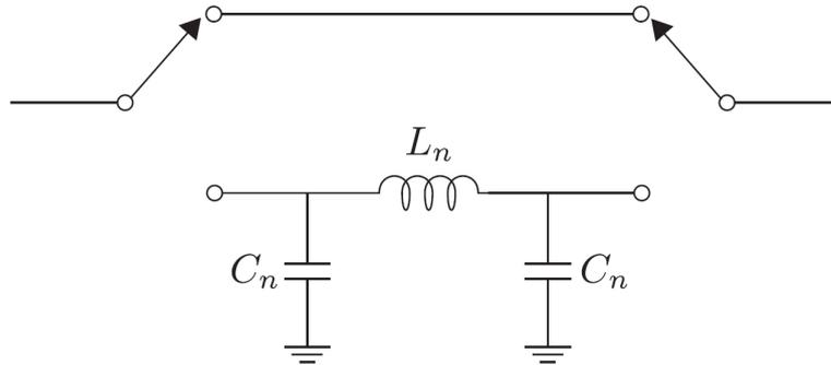
**Figure 16:** By-pass/Low-pass phase shifter [4]
