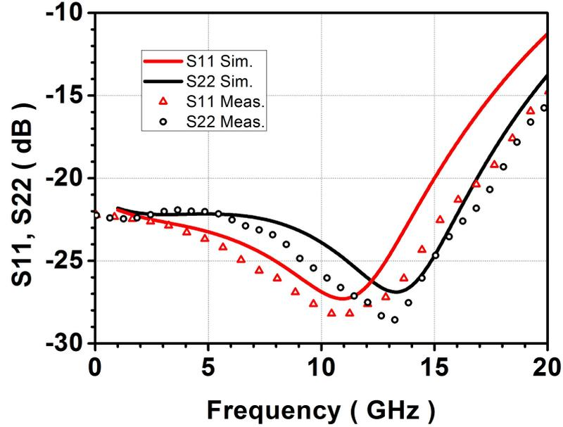
**Figure 45:** Simulated and measured input/output return losses of the SPDT switch
