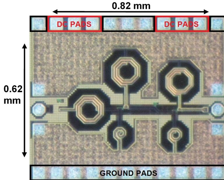
Figure 47: Chip photo of the fabricated LNA.
