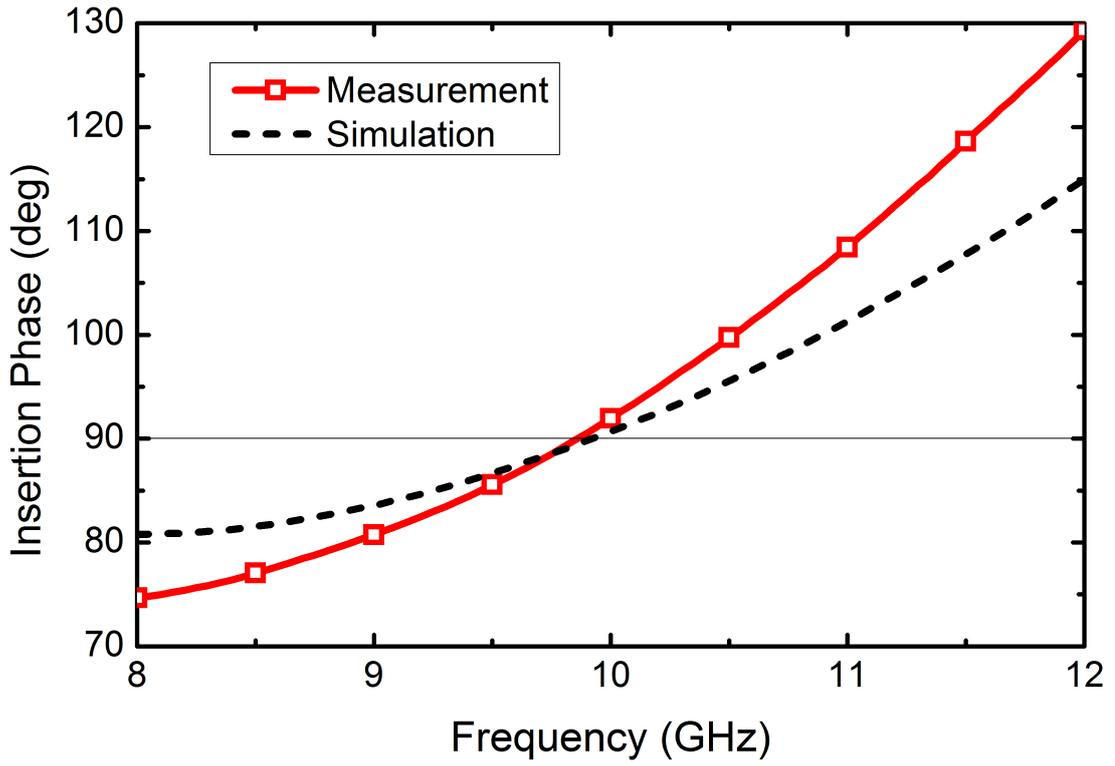
Figure 37: Simulated and measured phase shift of 90° bit.
