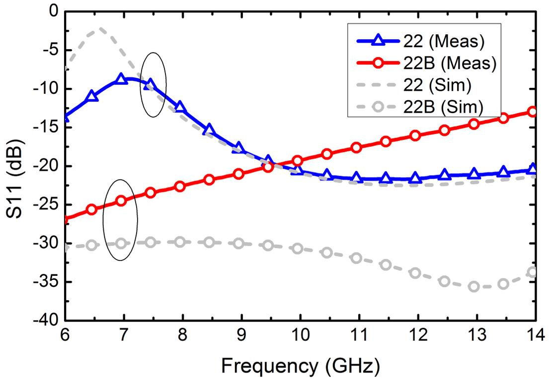
**Figure 26:** Simulated and measured return losses of 22.5° bit in both phase shift and bypass modes.
