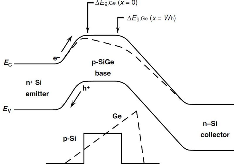
**Figure 9:** Energy band diagram of a Si BJT vs. SiGe HBT [1]
