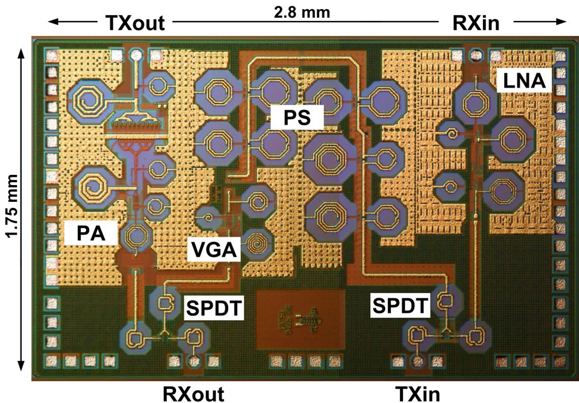
**Figure 54:** Chip photo of the fabricated SiGe X-Band T/R module. Chip size is  $4.9 \text{ mm}^2$ .
