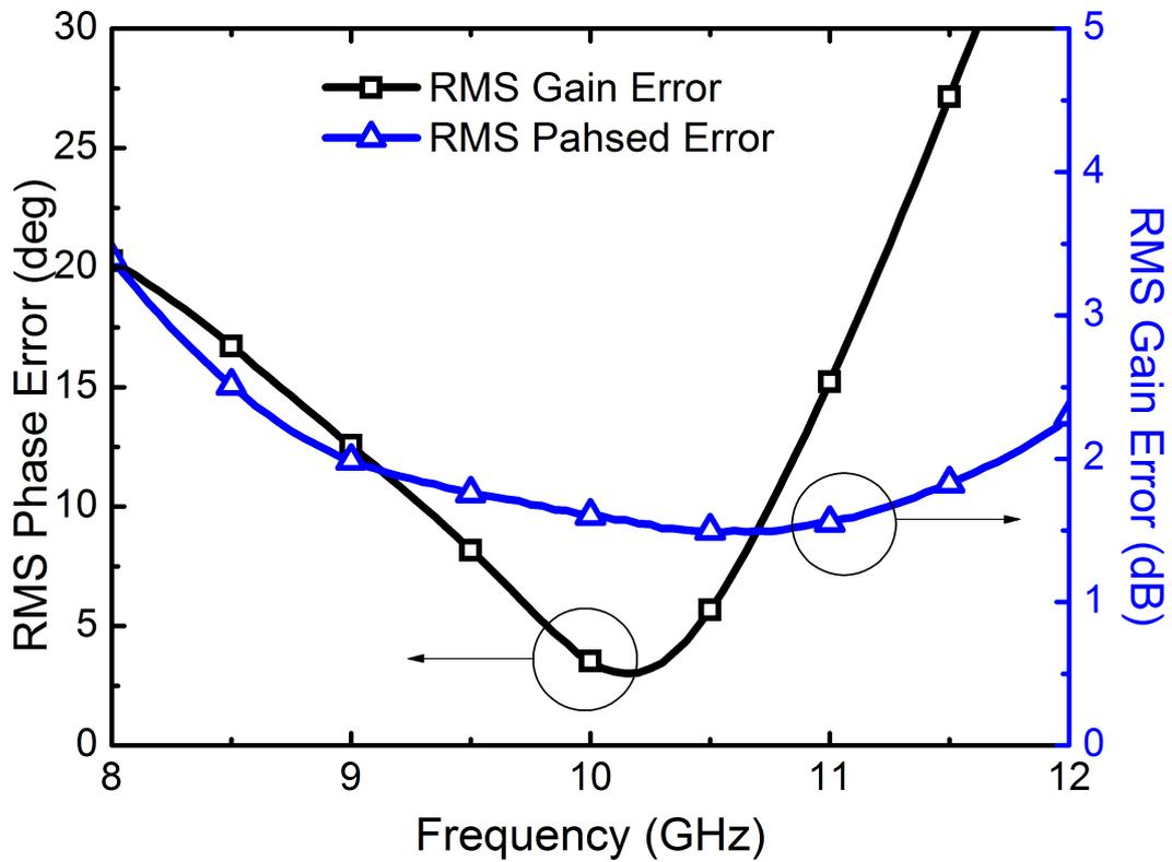
Figure 40: Measured RMS phase and gain error of 4-bit phase shifter.
