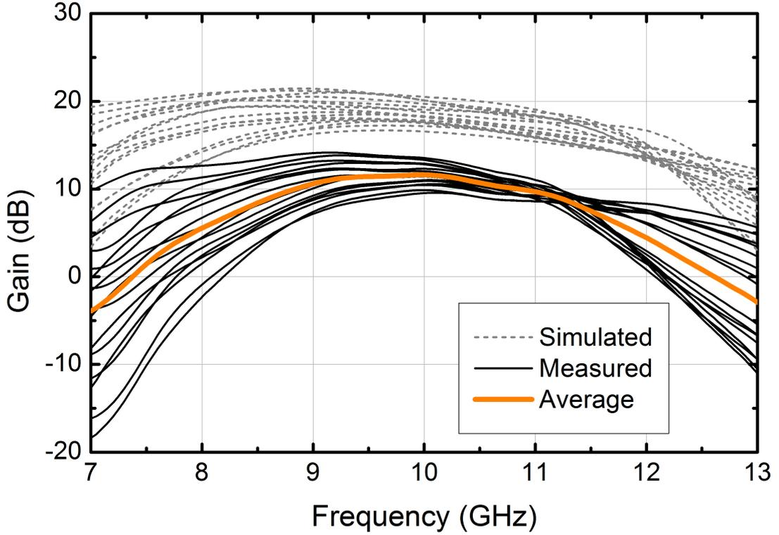
**Figure 58:** Simulated and measured gain of T/R module in receiver mode for all phase states
