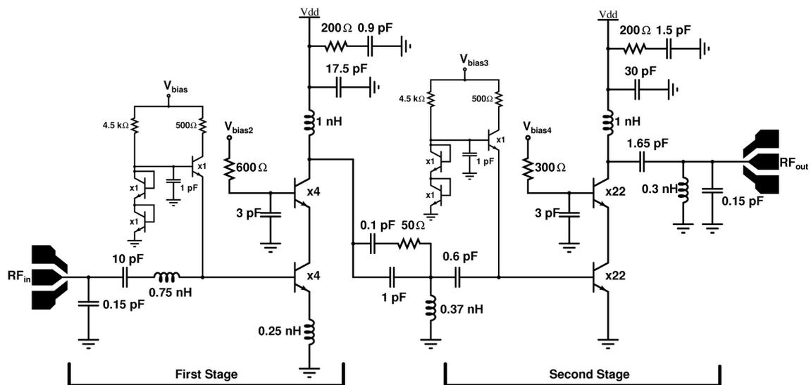
Figure 50: Schematic view of the two stage power amplifier.
