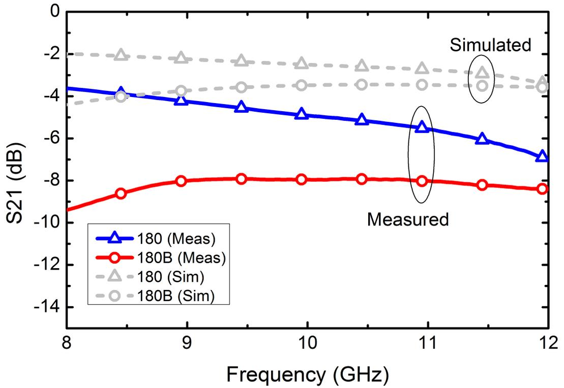
**Figure 33:** Simulated and measured insertion losses of 180° bit in both phase shift and bypass modes.
