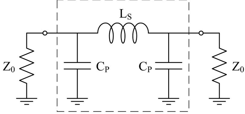
**Figure 20:** Schematic view of  $\Pi$ -type low pass filter
