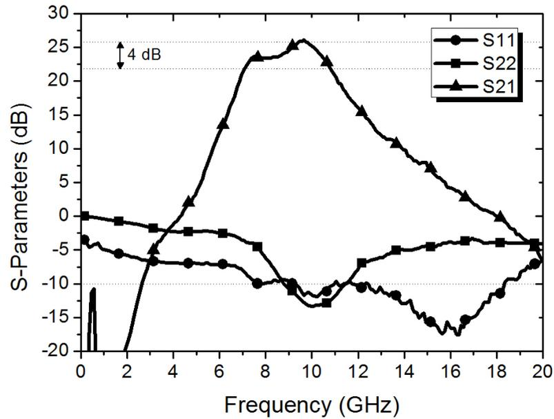
**Figure 52:** Measured gain and return losses of the PA.
