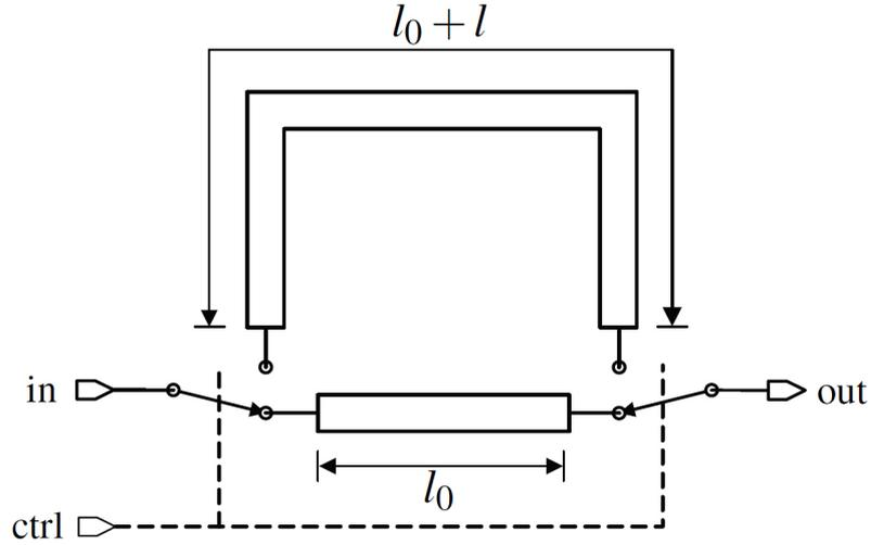
**Figure 12:** Switched-line phase shifter [3]
