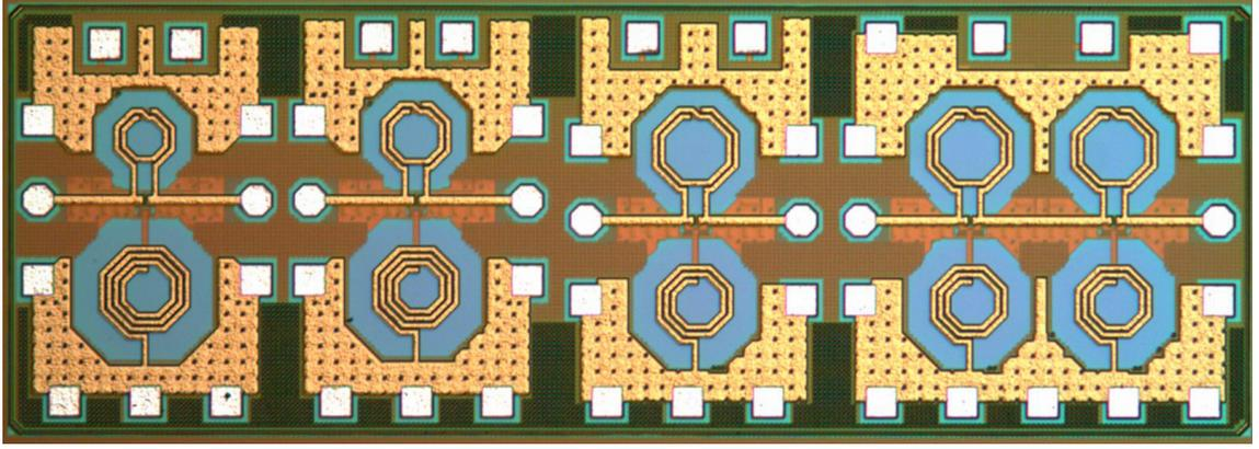
**Figure 25:** Chip photo of the fabricated 4-bit SiGe X-band passive phase shifter.
