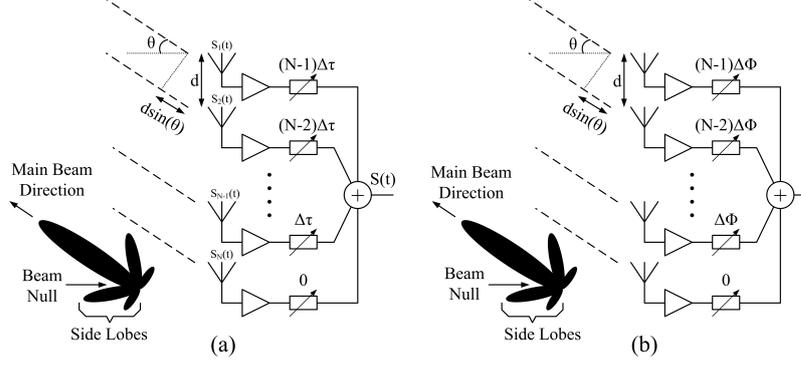
**Figure 2:** Basic timed-array receiver block diagram.
