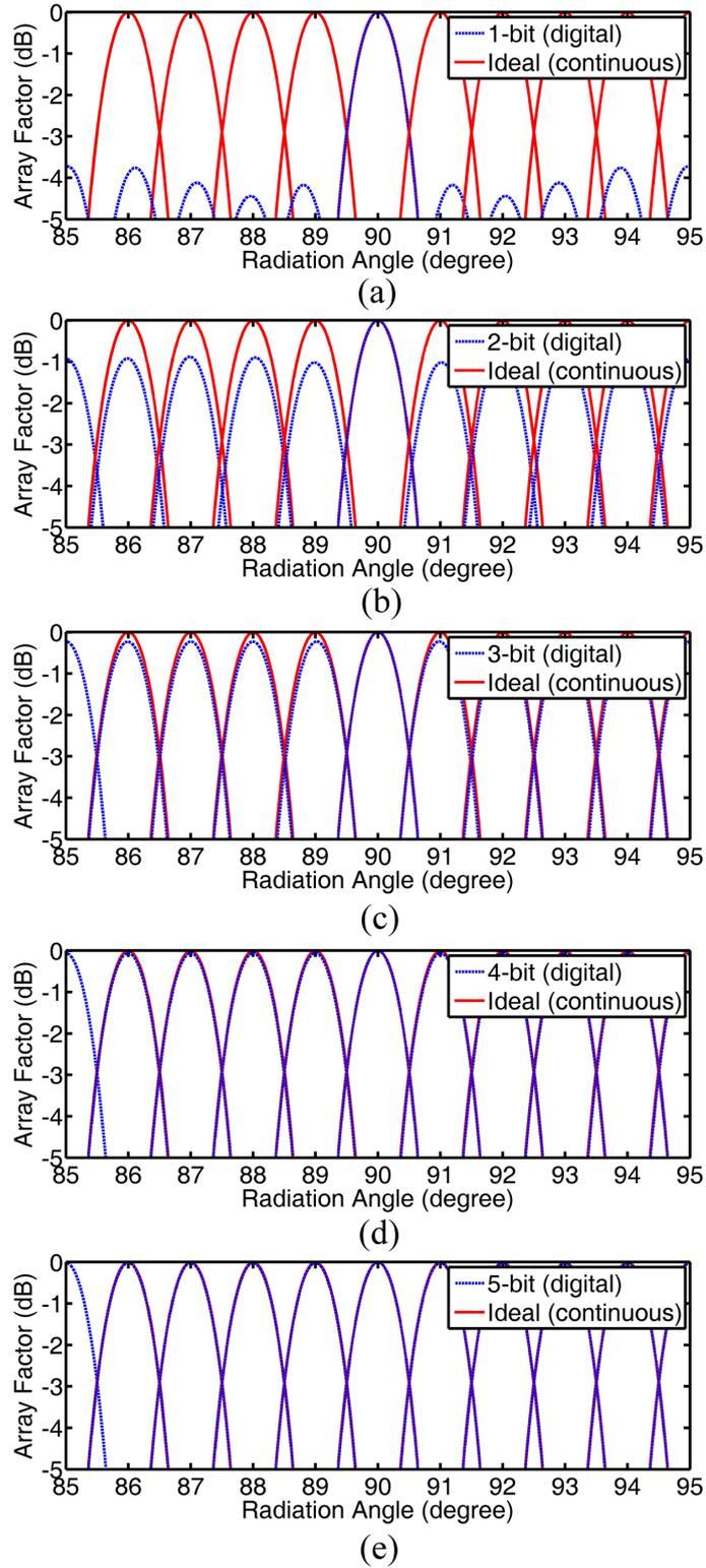
**Figure 18:** Comparison between continuous phase shift and discrete phase shift, displaying quantization loss. Figures show normalized array factors of a linear array with  $N=100$  elements and  $\lambda/2$  spacing, using (a) 1-bit (b) 2-bit (c) 3-bit (d) 4-bit (e) 5-bit digital phase shifting. Quantization loss is negligible after 4-bits.
