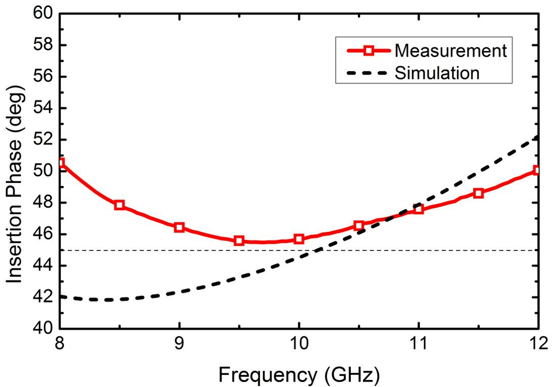
**Figure 36:** Simulated and measured phase shift of 45° bit.
