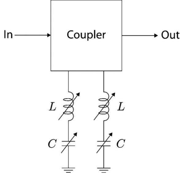
**Figure 14:** Reflection type phase shifter [4]
