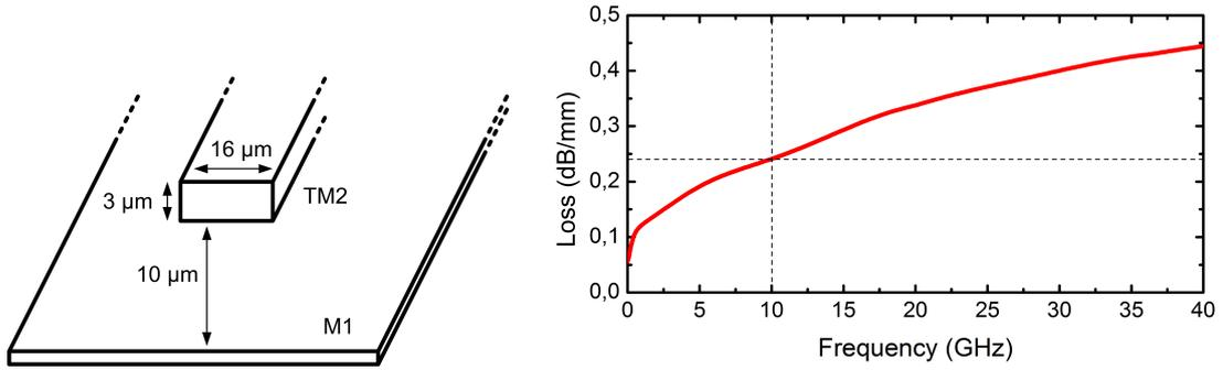
**Figure 55:** (a) Designed microstrip transmission line in SiGe BiCMOS process
