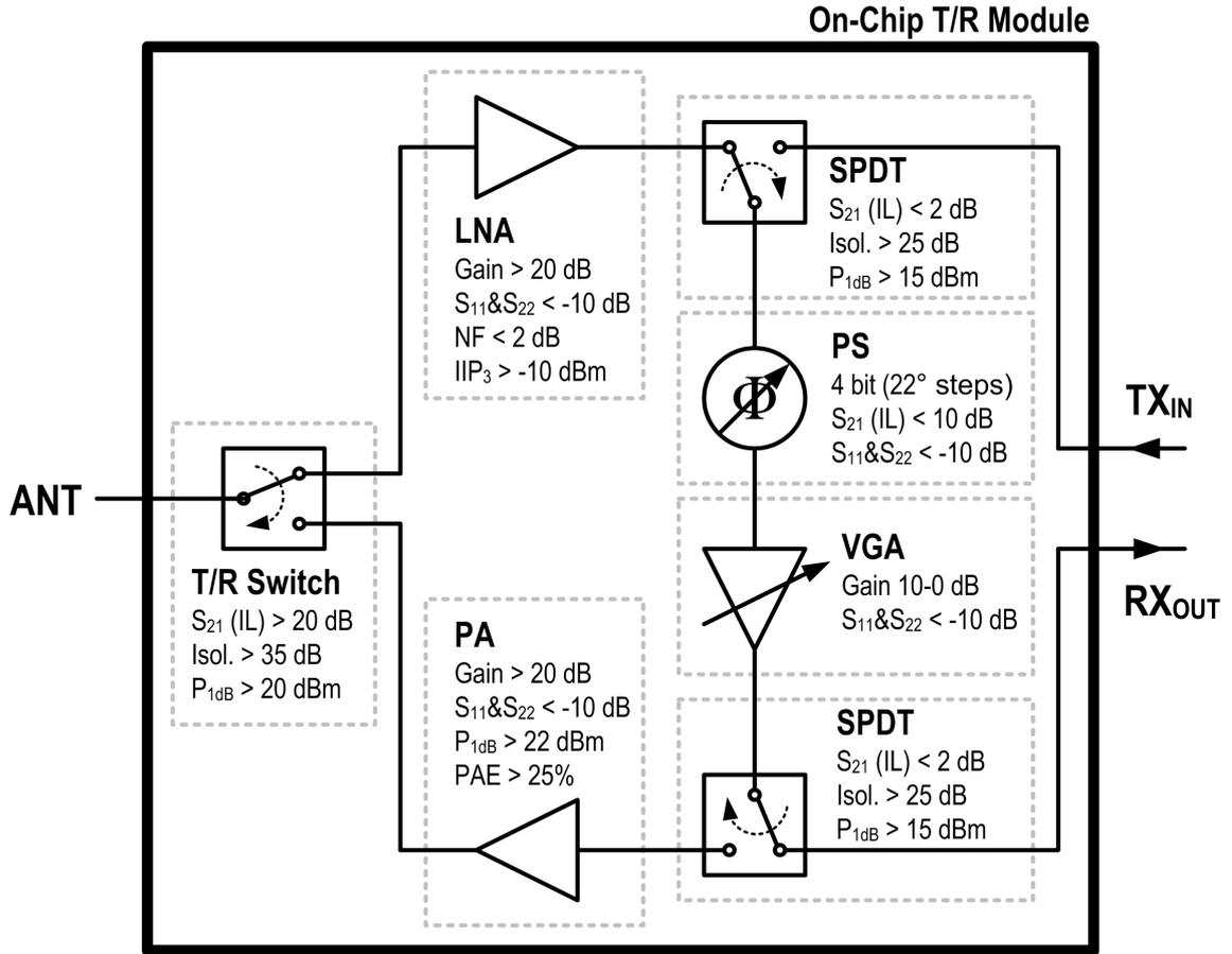
**Figure 11:** SiGe X-band all-RF T/R module block diagram and component specifications
