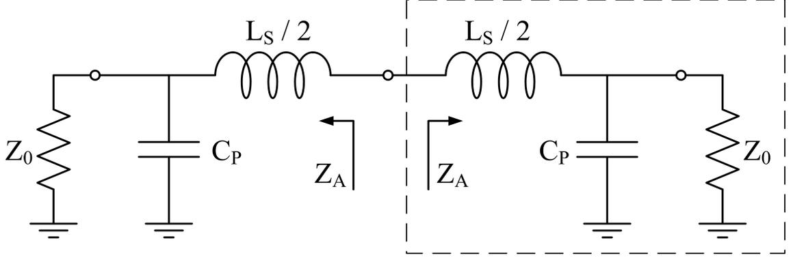
**Figure 21:** Decomposition of  $\Pi$ -type low-pass filter into two symmetric circuits
