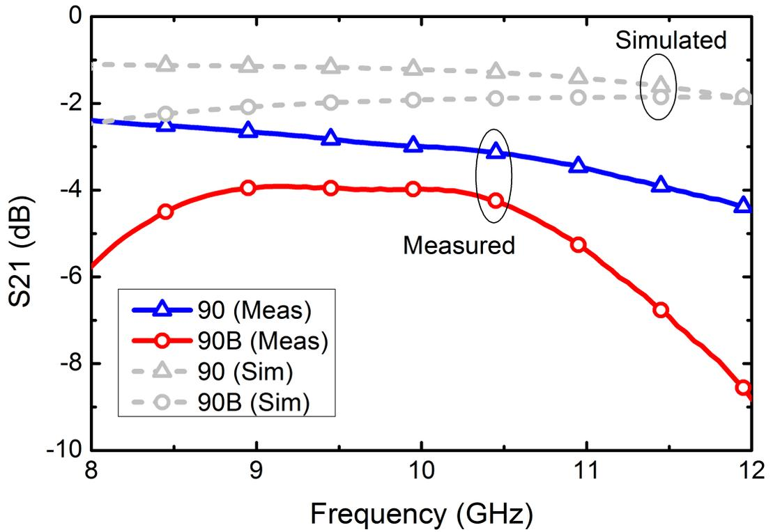
**Figure 32:** Simulated and measured insertion losses of  $90^\circ$  bit in both phase shift and bypass modes.
