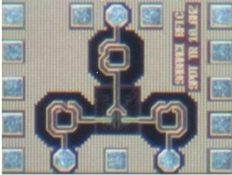
**Figure 43:** Chip photo of the SPDT switch. Chip area is  $0.48 \times 0.36 \text{ mm}^2$
