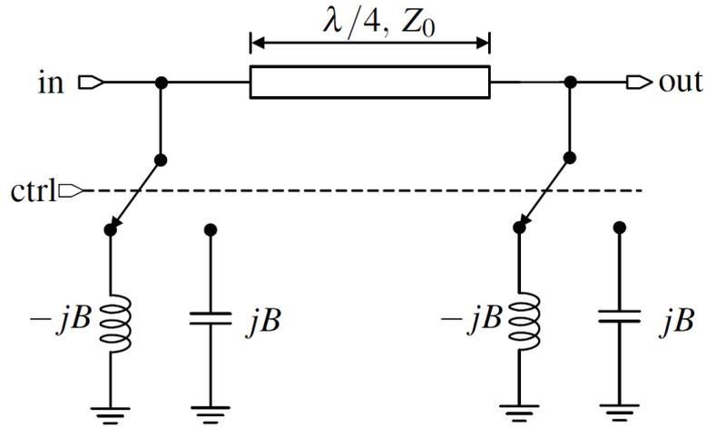
**Figure 13:** Loaded-line phase shifter [3]
