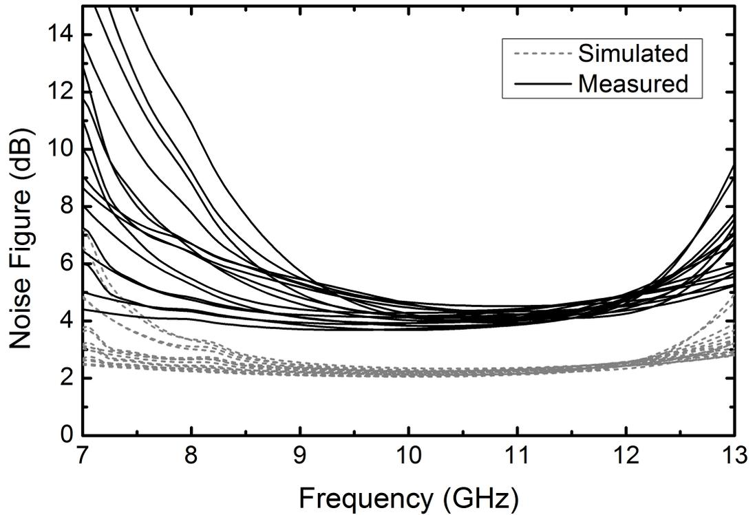
Figure 60: Simulated and measured noise figure of T/R module in receiver mode
