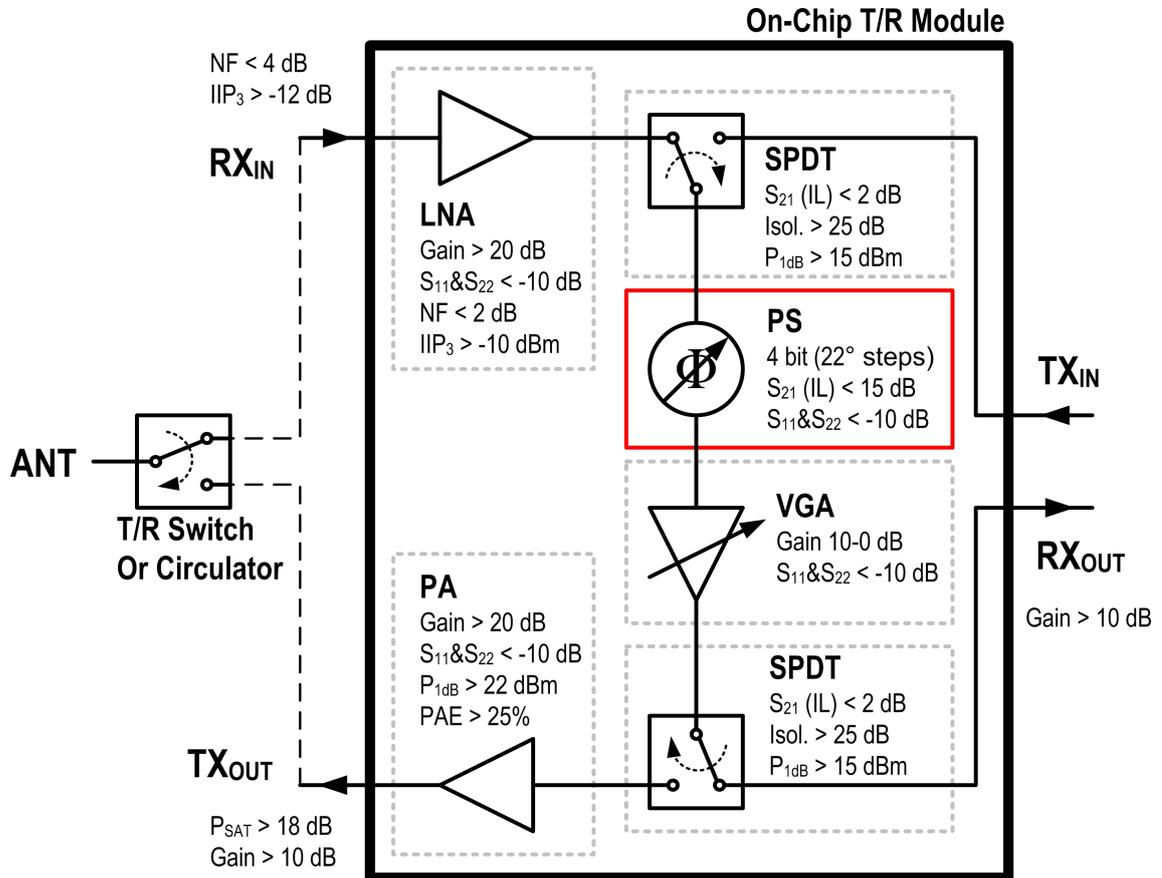
**Figure 41:** Proposed SiGe X-Band T/R Module Architecture
