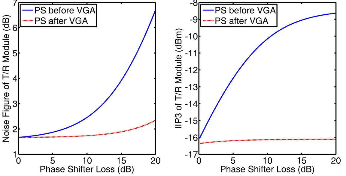
**Figure 68:** Simulated noise figure and third order intercept point of T/R module vs. phase shifter loss, using measured results of other building blocks.
