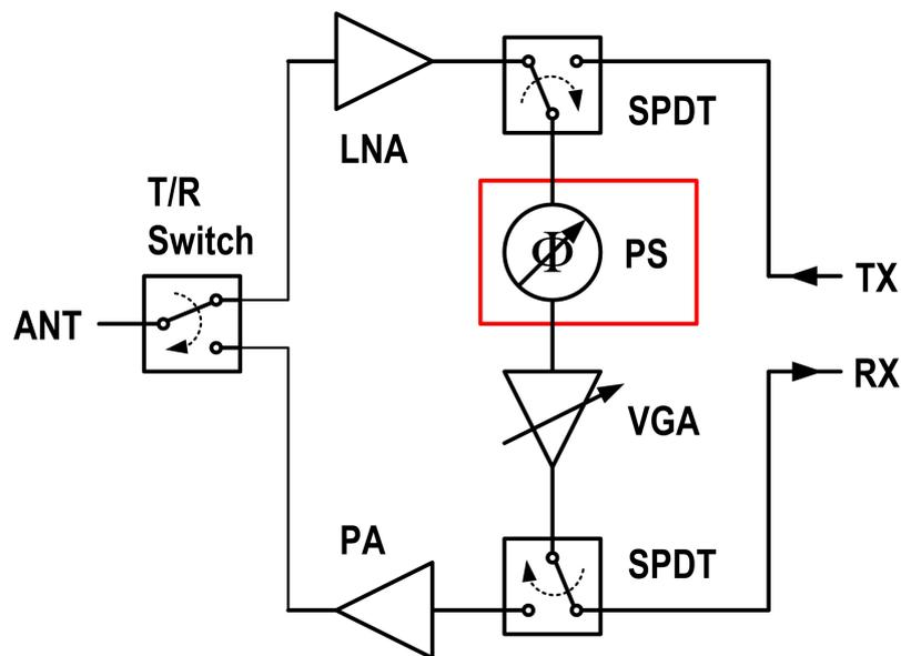
Figure 19: System diagram of a T/R module
