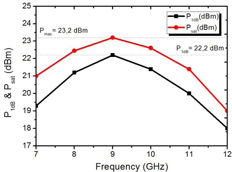
**Figure 53:** Measured 1-dB compression point and saturated output power of the PA.
