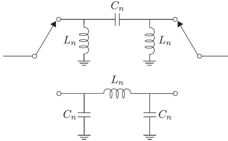
**Figure 15:** High-pass/Low-pass phase shifter [4]
