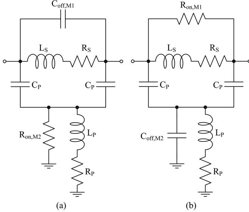
**Figure 24:** Equivalent circuit schematics for the phase shifter in (a) phase shift mode and (b) bypass mode, including inductor parasitics
