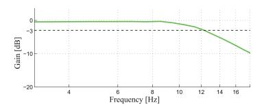
Fig. 3. Velocity control bandwidth
