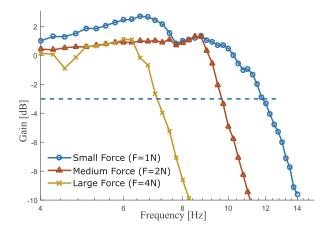
Fig. 4. Bode magnitude plots characterizing small, medium, and high force bandwidths
