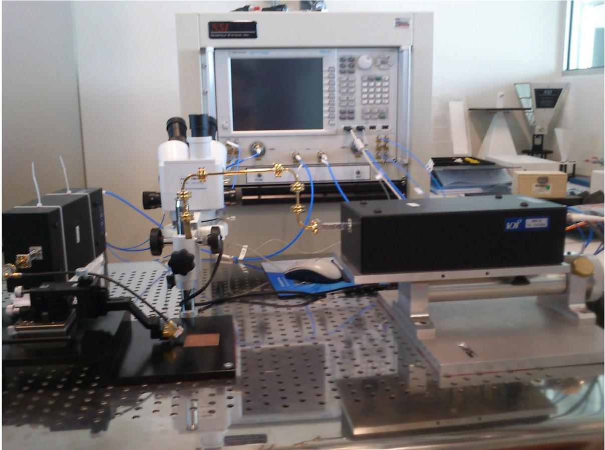
Fig. 4.2 Implemented Millimeter Wave Antenna Setup
