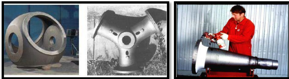
Figure 3.2: Different wind turbine components with ductile iron configurations (9).
