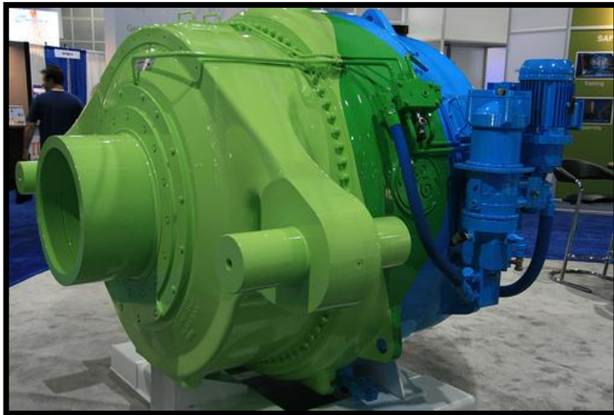
Figure 1.7: Standard 3 stage gear box for a middle class wind turbine (7).
