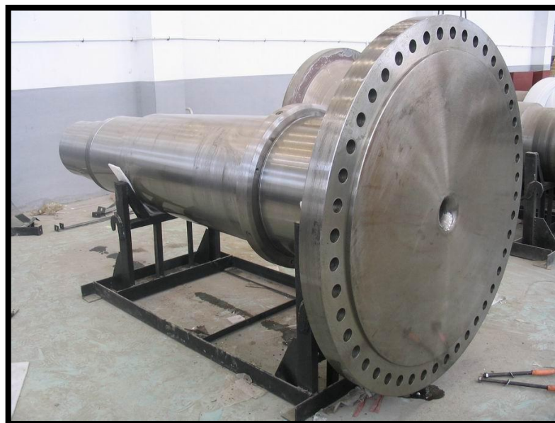
Figure 1.6: The low speed shaft for a wind turbine (6).
