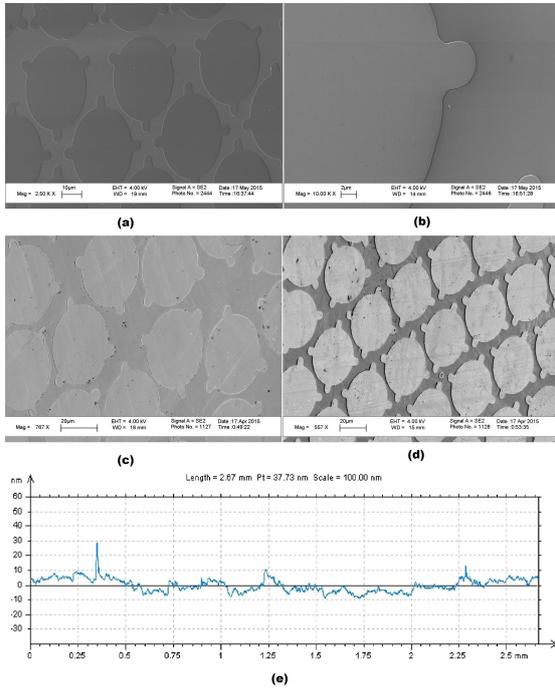
Fig. 2. (a) Sacrificial grooves on Silicon wafer, (b) Sacrificial Chromium with negative offset leveling, (c) Almost leveled ( $\pm 10$  nm positive offset) sacrificial patterns, (d) Patterns with considerably higher positive offset, (e) Profilometric measurement showing less than 10 nm step difference between patterns and Silicon surface after sacrificial patterning.
