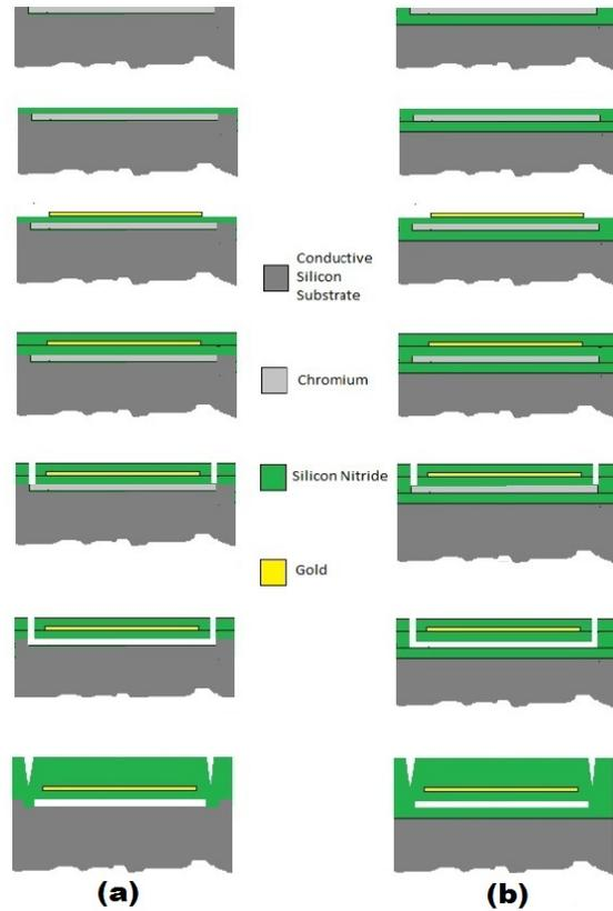
Fig. 3. Process flow for (a) Sacrificial grooves on Silicon wafer, (b) Sacrificial grooves on insulating Silicon Nitride coating on Silicon
