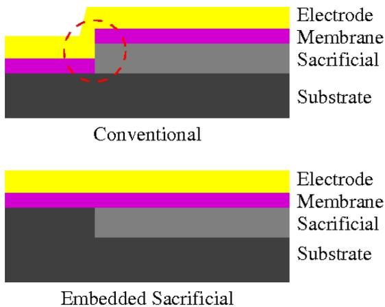
Fig. 1. The conventional fabrication method requires a first silicon nitride layer to be atleast as thick as the sacrificial to separate the device electrode from the sacrificial layer. A nonconformal thinner layer produces a profile as marked by the circle in the upper plot. The proposed method alleviates this problem by embedding the sacrificial layer.
