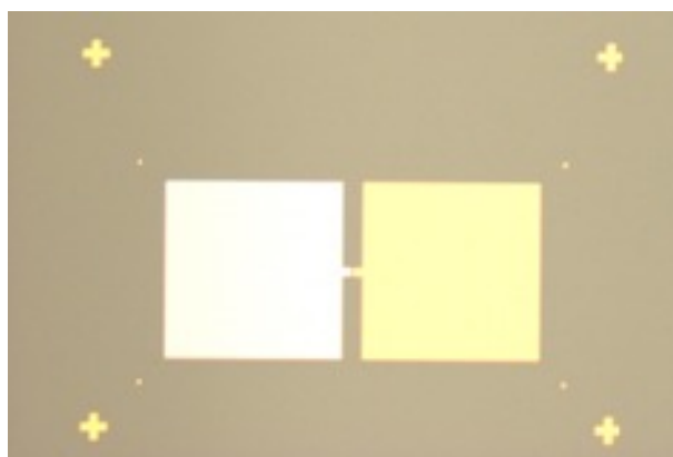
Figure 3 - Optical microscopy images of the fabricated diodes.
