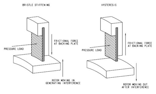
Figure 5: Role of friction in seal stiffening [5].
