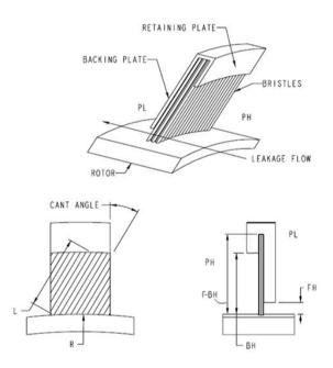
Figure 1: Brush seal schematic and main design parameters.
