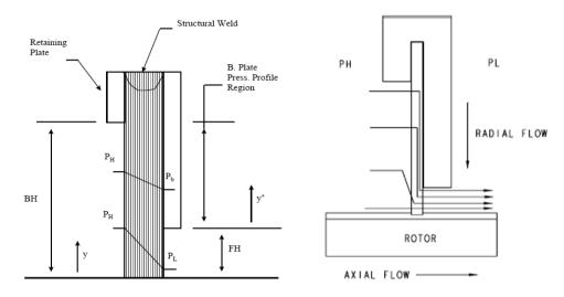
Figure 6: Brush seal internal pressure distribution and leakage flow through the bristle pack [5].
