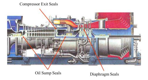
Figure 13: Typical brush seal application areas in a gas turbine.
