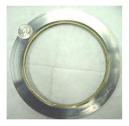
Figure 2: Aramid brush seal prototype [4].
