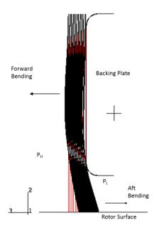
Figure 8: Brush pack behavior under pressure load [5].
