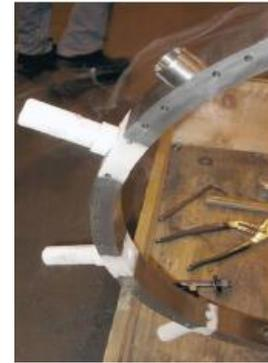
**Figure 2.3** – Shrink-fit method
