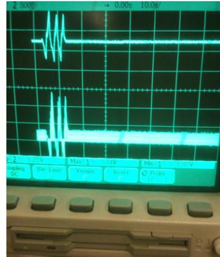
**Figure 3.9** – Comparison of filtered and unfiltered load cell signals via oscilloscope.
