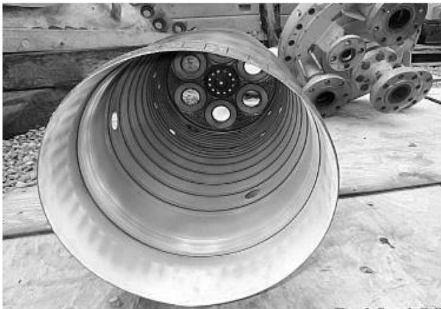
Figure 1.4 – Combustion can [4]
