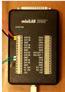
Figure 3.10 – miniLAB 1008 10 bit data acquisition card.
