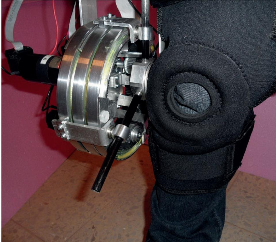
Figure 3.2: The isometric view of the exoskeleton prototype attached to knee.
