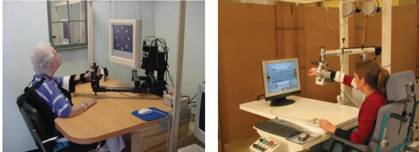
Figure 1.3: Fixed based upper limb rehabilitation robots: MIT-Manus and Gentle/s respectively
