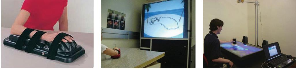
Figure 1.4: Mobile upper limb rehabilitation robots: Arm-skate, Rutgers arm and system with Wii remote respectively
