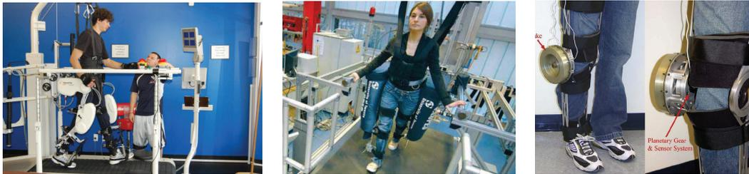
Figure 1.1: Lower limb rehabilitation robots: Lokomat, Lopes and ERF knee respectively
