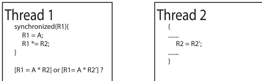
Figure 2: An **atomicity violation** example where programmer assumes synchronizing R1 in Thread 1 will secure the atomicity of the operation. Eventhough the lock is held, a concurrently running thread, Thread 2, may change the contents of the shared resource R2.
