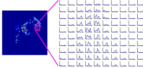
Fig. 6. Anisotropy characterization for a subset of pixels in the backhoe loader using joint subaperture reconstruction imposing piecewise smoothness in angular scattering. The individual small plots on the right have subaperture angle  $\hat{\theta}$  as the abscissa and the scattering magnitude  $|s(\hat{\theta})|$  as the ordinate. They are arranged to match the pixel locations in the image on the left.
