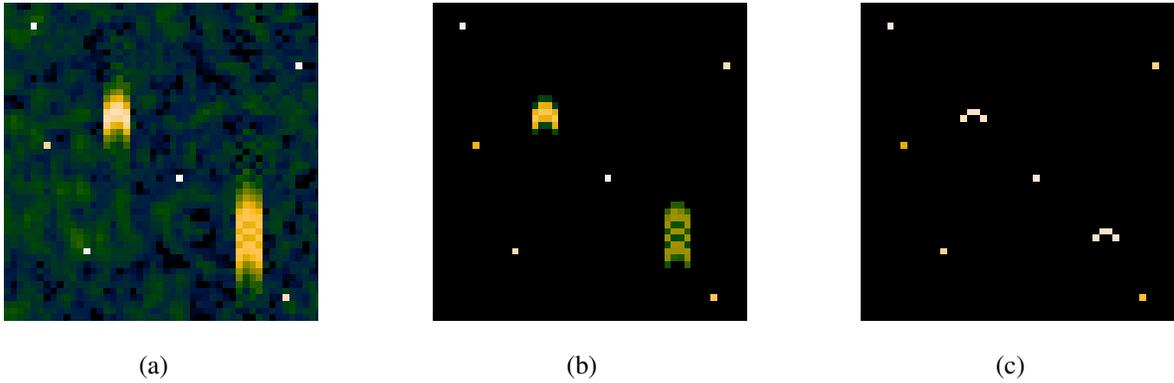
Fig. 10. Imaging of a synthetic scene with moving targets. (a) Conventional imaging. (b) Sparsity-driven imaging assuming a stationary scene. (c) Joint sparsity-driven imaging and phase error correction.
