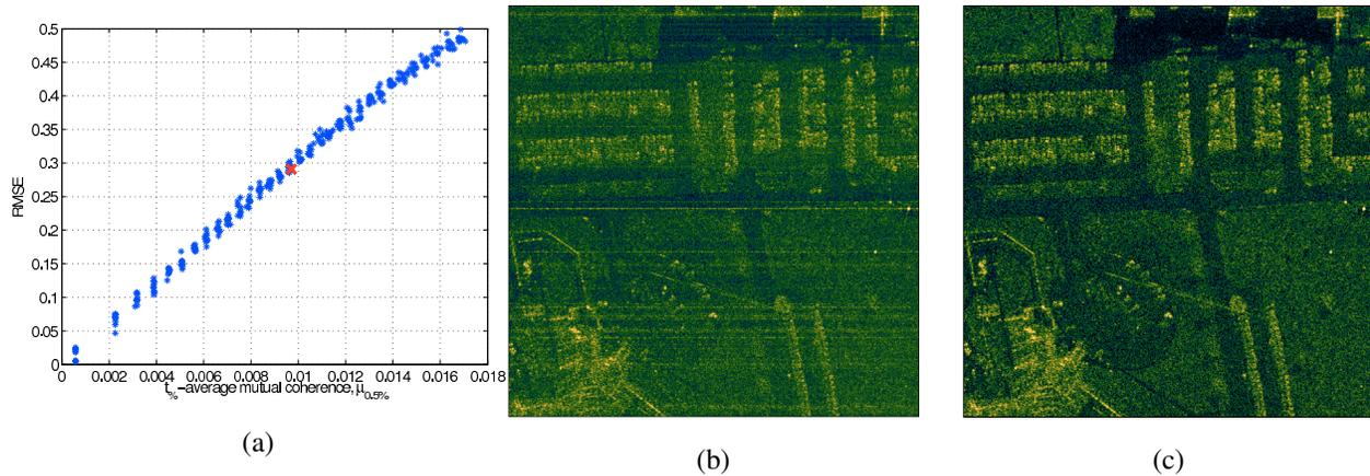
Fig. 8. Compressed sensing based analysis of sensing configurations. (a) RMSE vs.  $\mu_{0.5\%}$ . (b) Conventional reconstruction, and (c) Sparsity-driven reconstruction corresponding to the red point in (a) with 24% of missing data [43].
