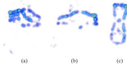
Fig. 4. Sparsity-driven 3D SAR imaging of a car. (a) 3D view. (b) Side view. (c) Top view. (To be used in the final paper after obtaining permission [27].)
