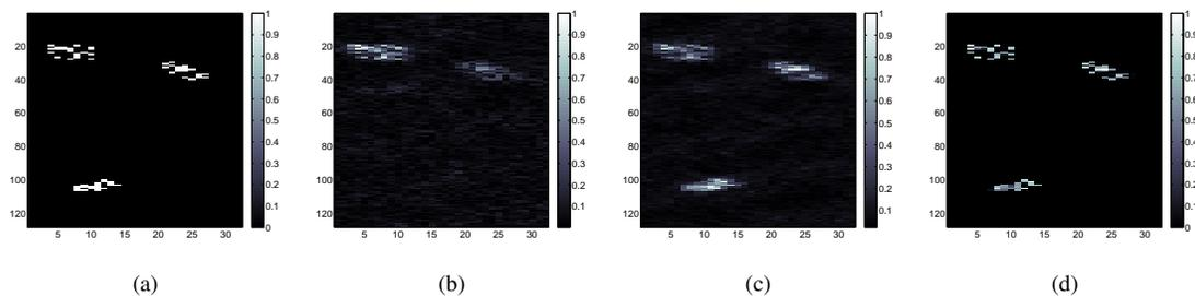
Fig. 9. Multistatic moving target imaging. (a) Simulated ground truth scene at time  $t = 0$ . The upper left target is stationary, the upper right target moves slowly, and the bottom target moves at a faster velocity. (b) Conventional reconstruction when motion is ignored. (c) Conventional reconstruction over a set of velocity hypotheses. (d) Sparsity-enforcing overcomplete dictionary reconstruction. Taken from [52].
