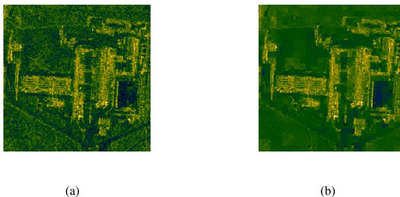
Fig. 2. Reconstructions of a scene based on TerraSAR-X data. (a) Conventional image. (b) Synthesis-based sparsity-driven image reconstructed using a multiresolution wavelet dictionary.
