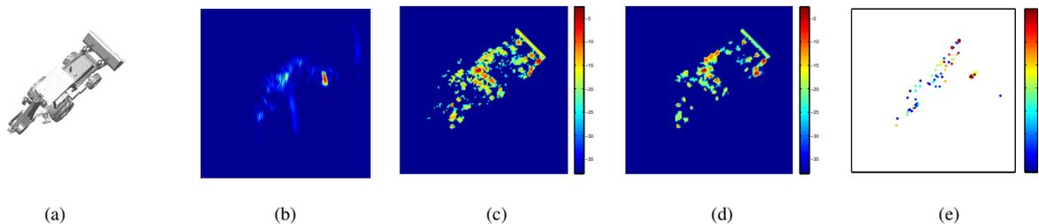
Fig. 5. Backhoe loader. (a) CAD model. (b) Conventional reconstruction. (c) Composite independent subaperture image. (d) Composite joint subaperture image imposing piecewise smoothness in angular scattering. (e) Composite joint subaperture image based on an overcomplete dictionary for angular scattering. Images taken from [30] and [29].
