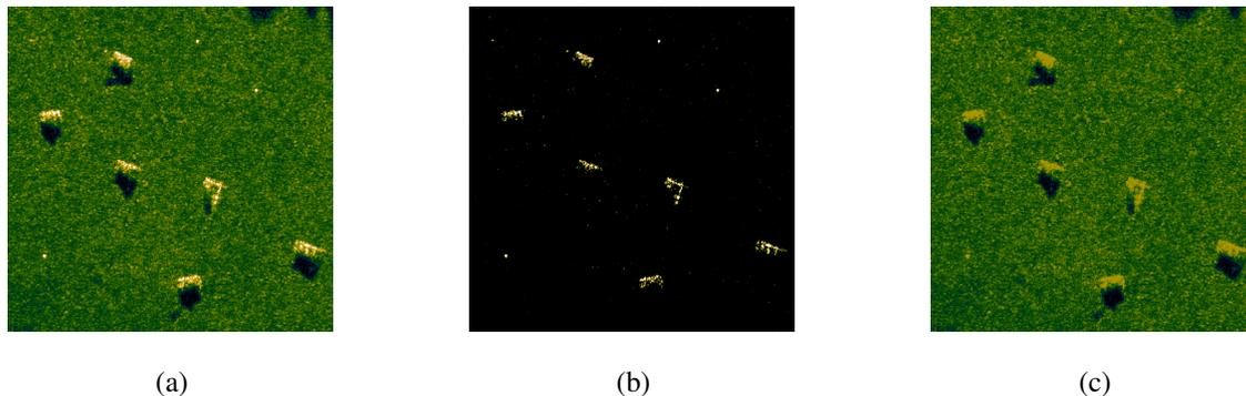
Fig. 3. Reconstruction of a scene from the MSTAR data set using a synthesis-based sparse representation approach combining the canonical (spike) dictionary with a learned dictionary. (a) Composite image. (b) Component consisting of strong scatterers represented by the spike dictionary. (c) Component represented by the learned dictionary.
