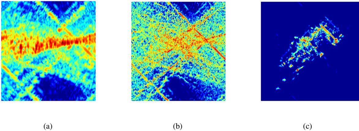
Fig. 7. Imaging in the presence of 1D phase errors uniformly distributed in  $[-\pi, \pi]$ . (a) Conventional imaging. (b) Sparsity-driven imaging without phase error compensation. (c) SDA: sparsity-driven imaging with phase error compensation.
