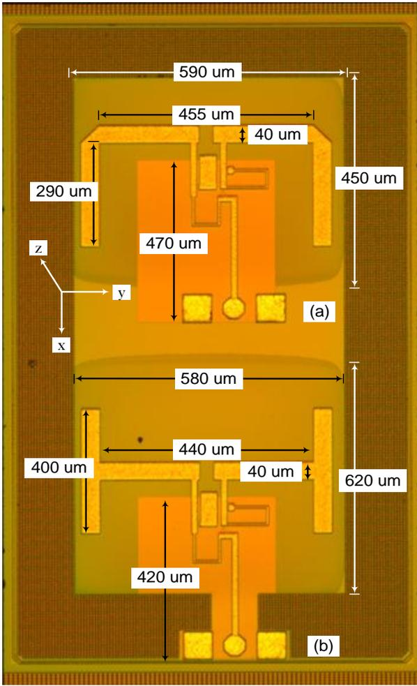
Fig. 1. Micrographic picture of the on-chip (a) L and (b) T shapes strip dipole antennas with different parameters size.
