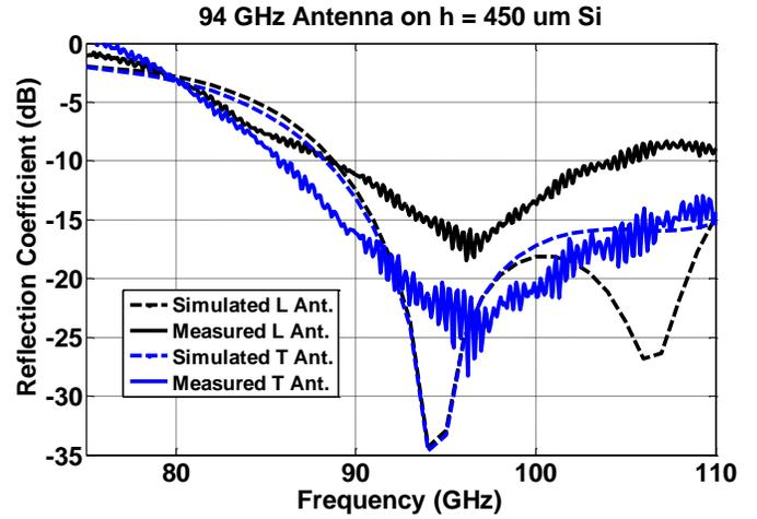
Fig. 2. Simulated and measured reflection coefficient for L and T shapes antennas.
