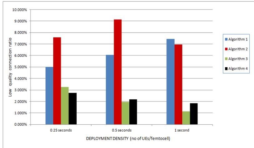
Figure 5.32: The ratio of active connections below  $E_c/I_o$  quality threshold of -18 dB
