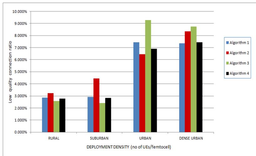
Figure 5.9: The ratio of active connections below Ec/Io quality threshold of -18 dB
