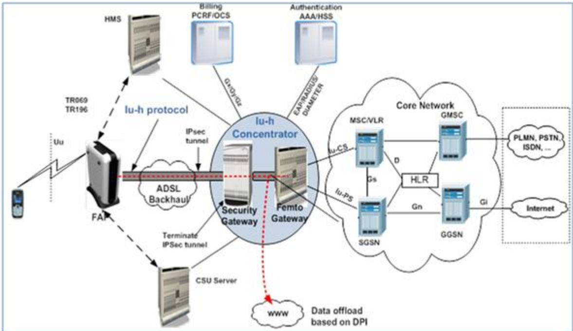
Figure 2.1: Femtocell solution architecture
