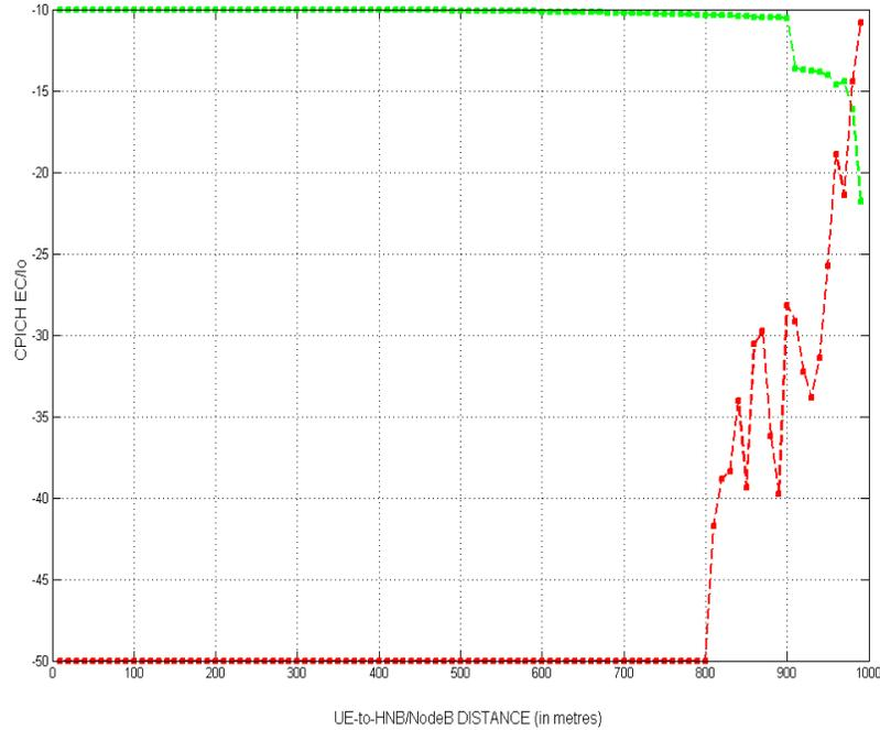
Figure 2.2: Sample diagram showing signal quality vs distance for HNB (red color) and NodeB (green color)
