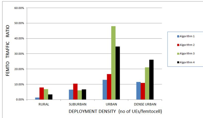
Figure 5.15: The ratio of CS traffic handled by femtocell network
