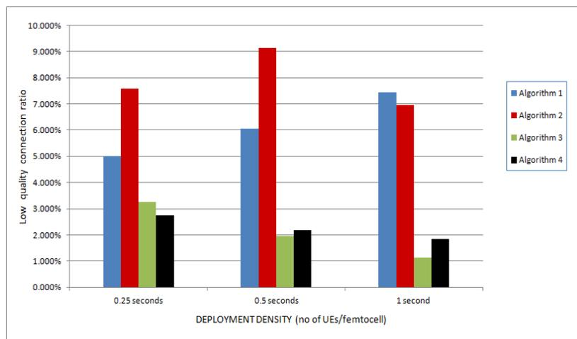
Figure 5.29: The ratio of active connections below  $E_c/I_0$  quality threshold of -18 dB
