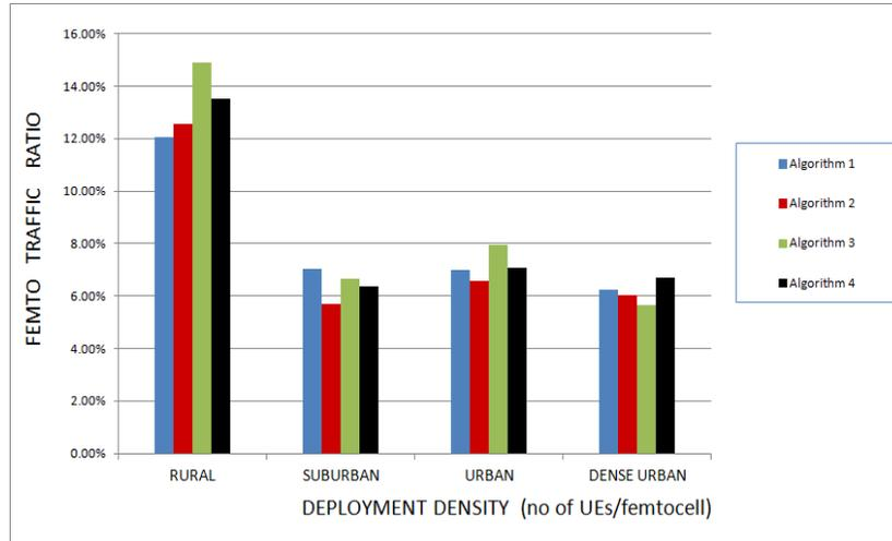
Figure 5.3: The ratio of CS traffic handled by femtocell network
