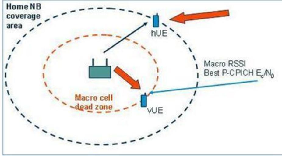
Figure 2.3: Femtocell SON algorithm operational criteria
