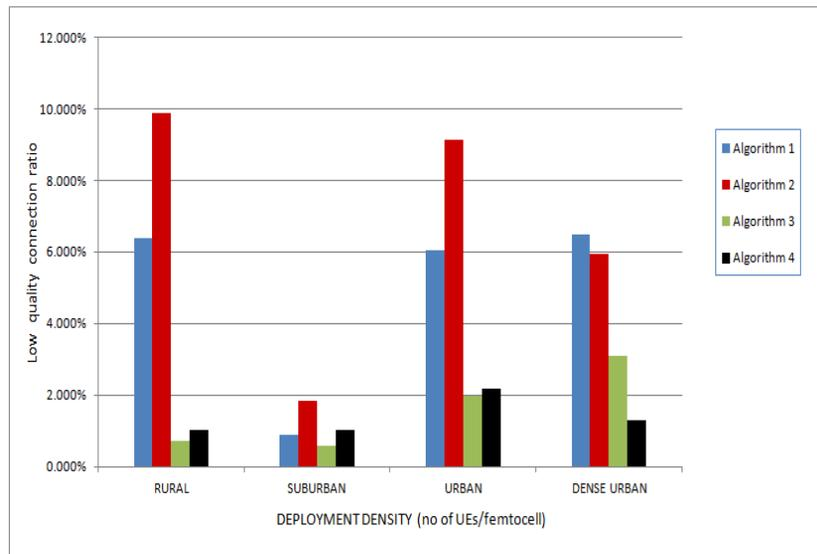
Figure 5.19: The ratio of active connections below  $E_c/I_o$  quality threshold of -18 dB
