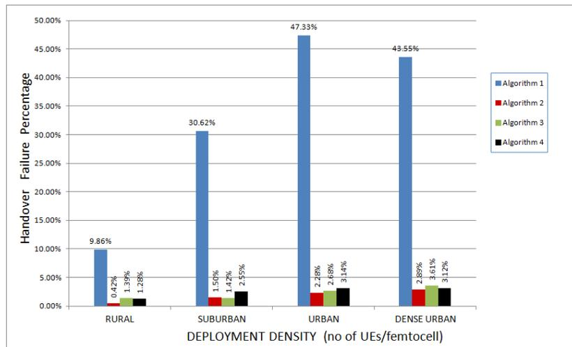
Figure 5.7: The percentage of HO failures
