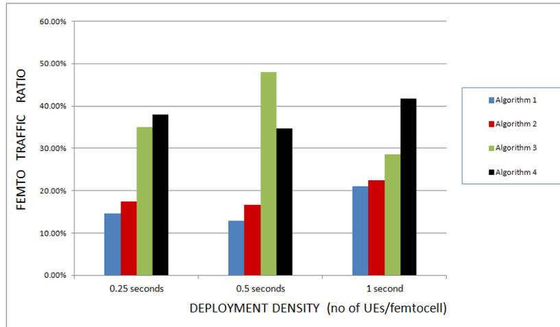
Figure 5.30: The ratio of CS traffic handled by femtocell network
