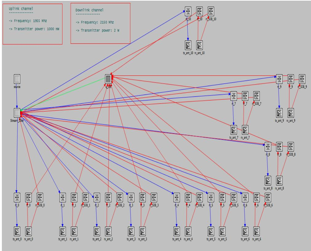
Figure 5.10: UE model in opnet that can support upto 10 scrambling codes
