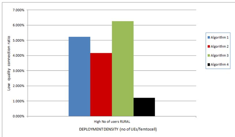
Figure 5.24: The ratio of active connections below  $E_c/I_o$  quality threshold of -18 dB
