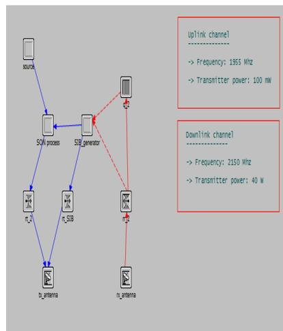
Figure 5.12: HNB/NodeB node model with SON processor and SIB packet generator
