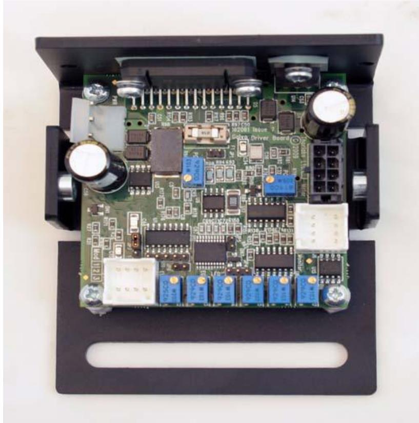
Fig. 3.20 Servo Driver Board
