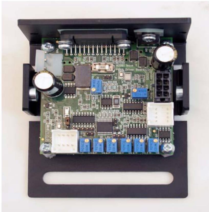
Fig. 3.20 Servo Driver Board
