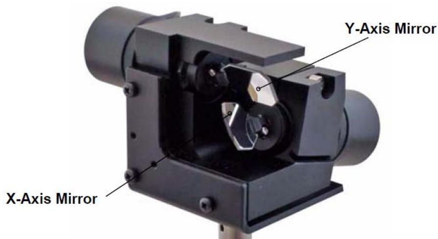
Fig. 3.6 Dual-axis Galvo Modules
