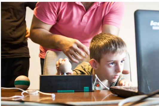
The game is played with a specially designed control device. A sphere object was used as the handler in this control device. The user can change the height of the bird by turning this sphere to right and left. Spheres of various sizes can be used and thus wrist and retention exercises of children living with
