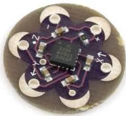
**Figure 3 - Accelerometer**
