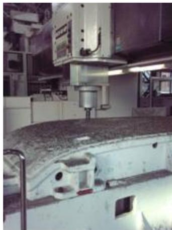
Figure 8.13 :Okuma 3-axis milling machine.
