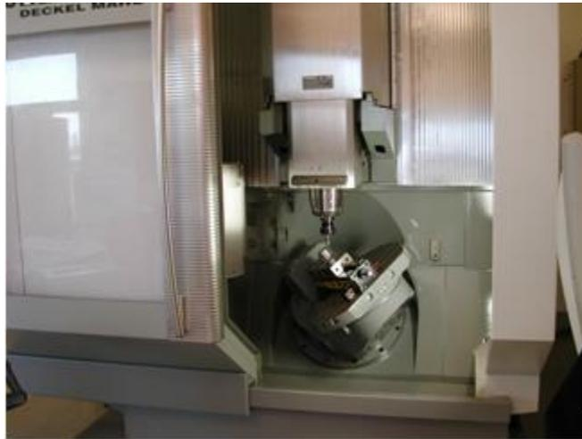
Figure 3.14: DMG 50 evolution 5-axis machining center
