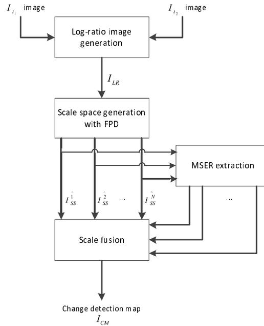
Figure 1: Overview of the proposed change detection algorithm.
