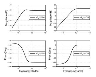
Fig. 5. Effect of %10 change in the nominal inertia on the estimation of acceleration. Mapping from input current is shown on the left column while mapping from disturbance is shown on the right column
