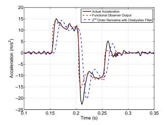
Fig. 10. Comparison of Accelerations from Functional Observer and Double Differentiation using Chebyshev 0.5dB Filter Under Constant Acceleration Reference
