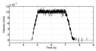
(b) Velocity Response of Filtered Differentiation using Butterworth filter
