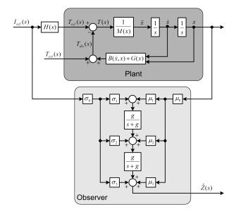
Fig. 3. Block diagram of functional observer
