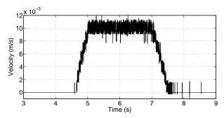
(a) Velocity Response of Filtered Differentiation using 2nd Order Low Pass Filter
