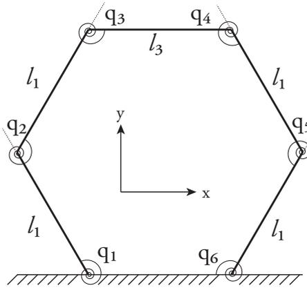
Figure 2.3: Pseudo-rigid body model of the half-pantograph mechanism
