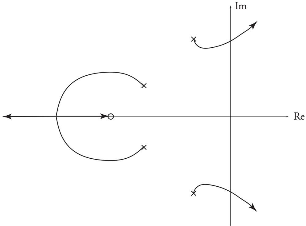
Figure 1.2: Root locus of the robotic manipulator with noncollocation.
