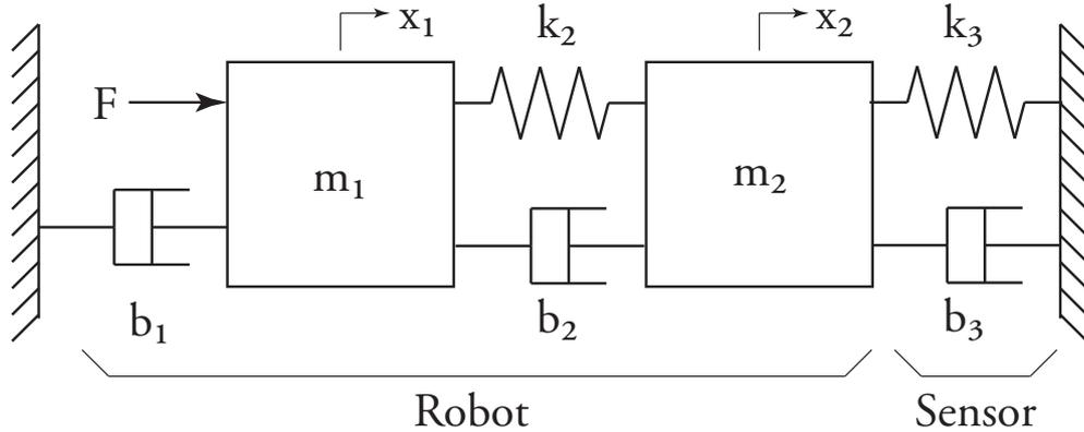
Figure 1.1: A robotic manipulator with a force sensor.
