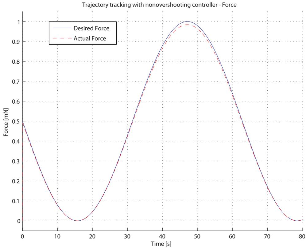
Figure 3.10: Sinusoidal force tracking of  $\mu$ SEA
