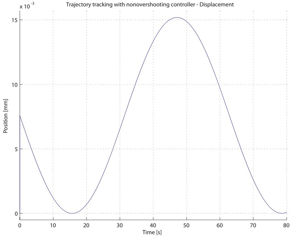
Figure 3.11: Displacement of the compliant coupling element of the  $\mu$ SEA in trajectory tracking
