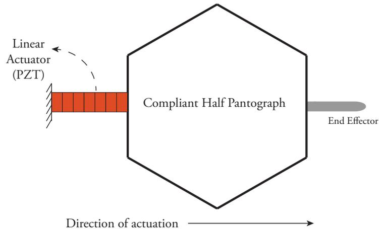
Figure 2.2: Schematic representation of the  $\mu$ SEA
