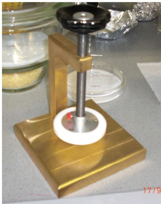
**Figure 2. 3: Press set-up used for PDMS pressing and other purposes.**
