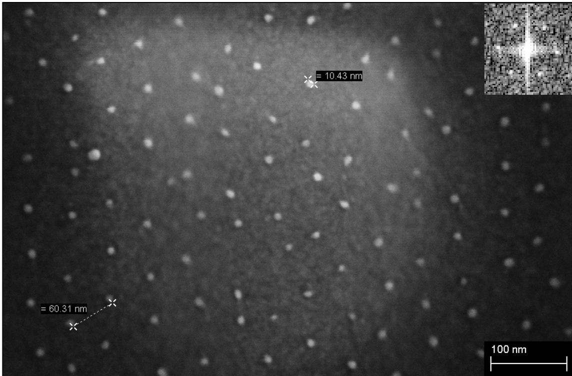
**Figure 3. 7: SEM image of LiOH and HF loaded micelles, spin coated on Si<sub>3</sub>N<sub>4</sub> substrate and etched with O<sub>2</sub> plasma after 15 hours of HF addition. FFT is given on the upper right corner**
