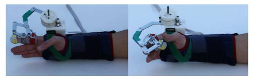
Figure 3.6: Tendon robot in extended and flexed configurations
