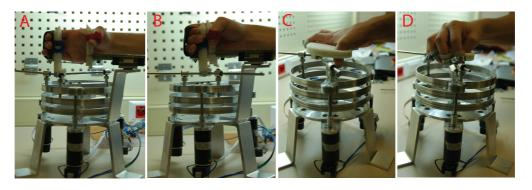
Figure 3.1: Specified motion imposing end effectors
