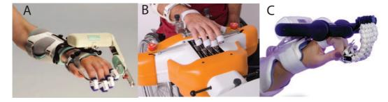
Figure 1.8: CPM type devices for hand therapy: (a)Hand 8091 (b)Amedeo (c)Maestra
