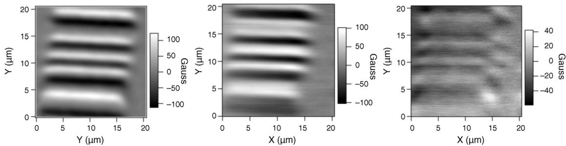
Figure 7.  $B_x$ ,  $B_y$ , and  $B_z$  images of a hard-disk sample surface obtained with 3D-SHPM (Dede, 2009).
