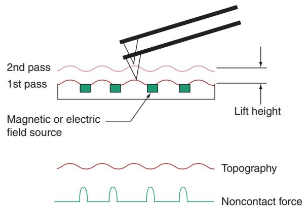
Figure 2. Lift-mode operation of MFM (Digital Instruments).
