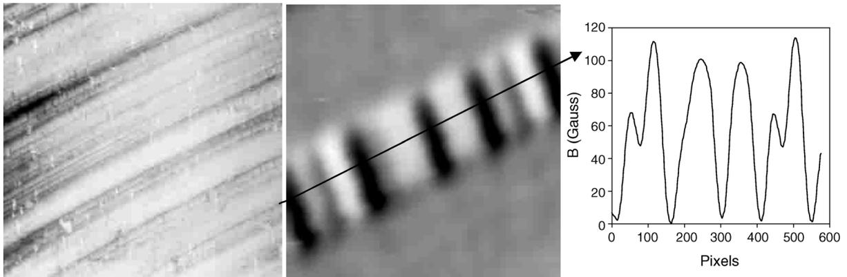
Figure 6. Topography,  $B_z$  image, and cross section of magnetic hard disk obtained by an SHPM image (Howells et al., 1999).
