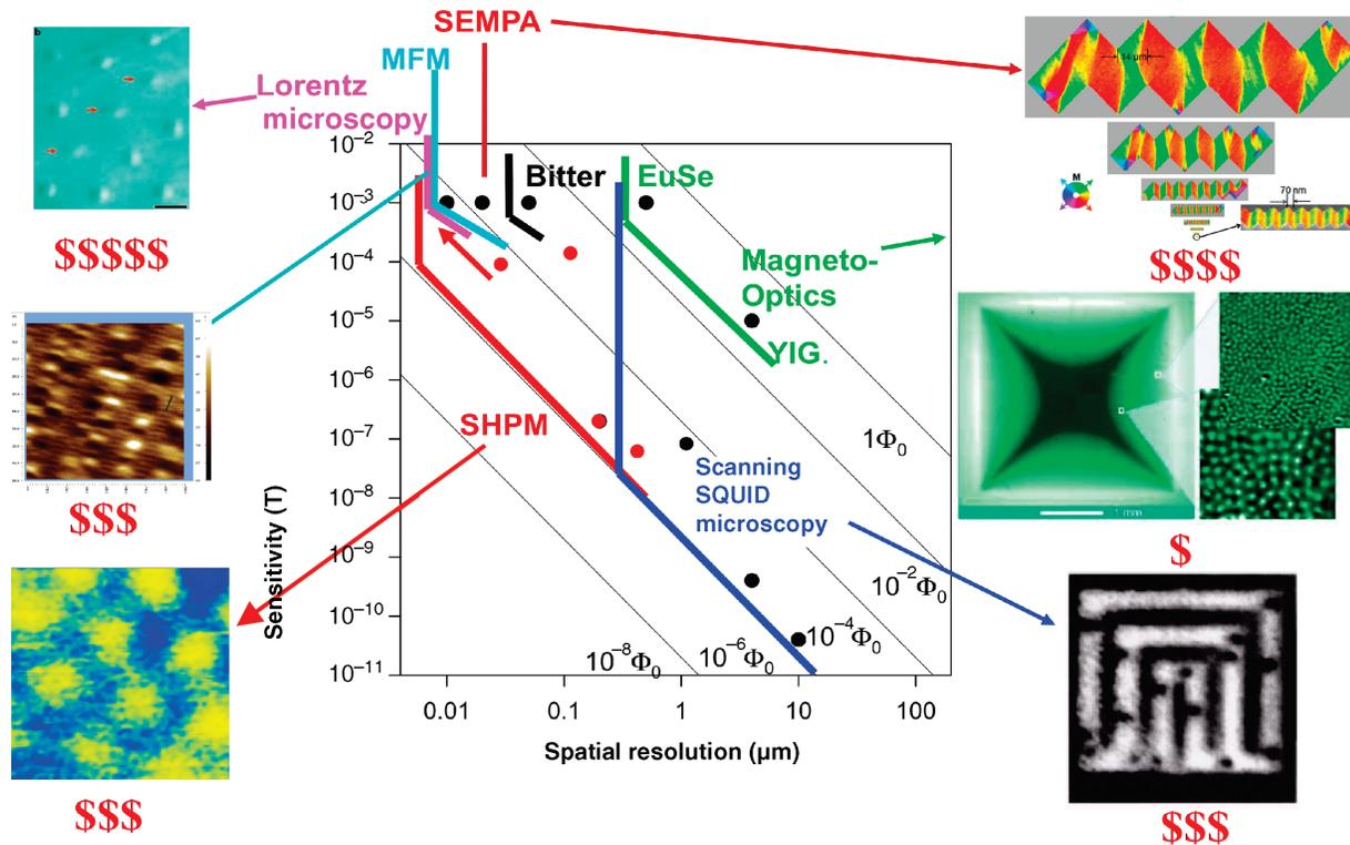
Figure 1. Comparison of magnetic imaging methods: magnetic resolution versus spatial resolution.
