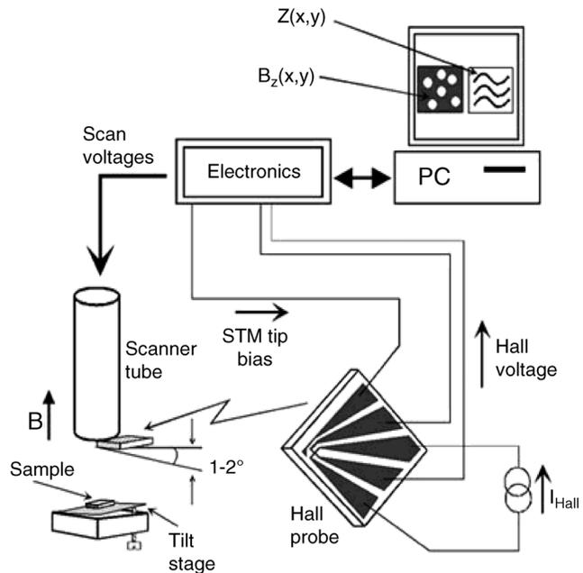
Figure 4. Principle of scanning Hall probe microscope (SHPM).
