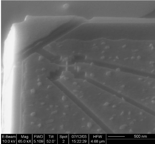
Figure 5. Bismuth thin film nano-Hall sensor integrated with an STM tip.
