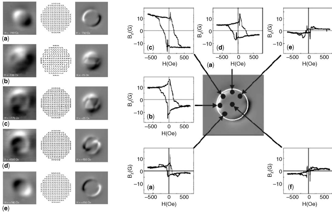
**Figure 8.** Local magnetization measurements performed on a 2 μm Fe disks using SHPM. Reprinted from (Neal et al., 2006), Copyright 2006, with permission from Elsevier.
