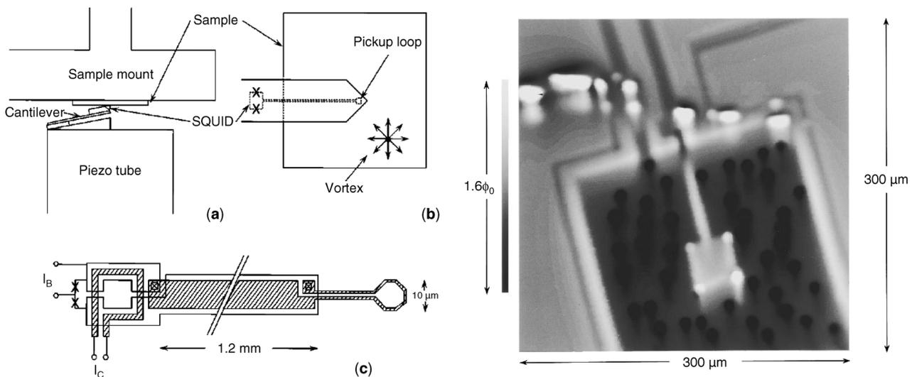
**Figure 9.** SSM and SSM image of a thin-film high- $T_c$  washer SQUID, with vortices trapped in the bulk of the washer, in a scratch in the SQUID, and at the inside corners of the square SQUID hole. Reprinted with permission from (Kirtley et al., 1995). Copyright 1995, American Institute of Physics.
