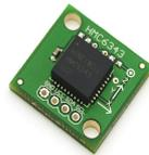
Figure 4.10: Tilt-compensated compass
