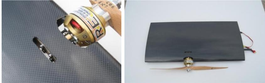
Figure 3.15: The finished wing with motor and motor driver
