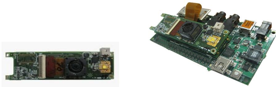
Figure 4.17: The camera solution for Gumstix
