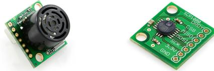
Figure 4.8: Sonar and barometric pressure sensor
