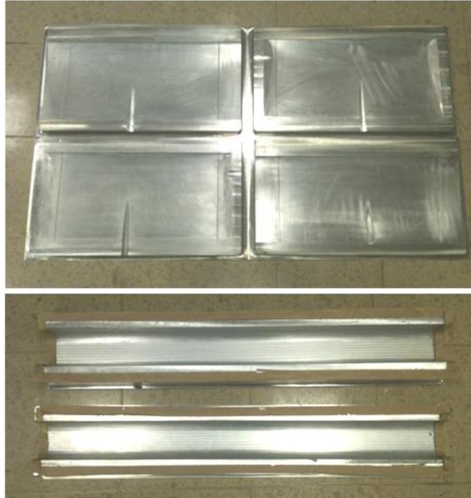
Figure 3.17: The CNC machined aluminum wing and fuselage molds
