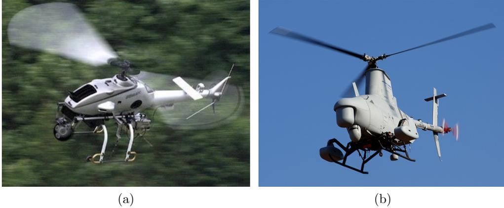
Figure 1.4: Yamaha RMAX (a) and Fire Scout (b)
