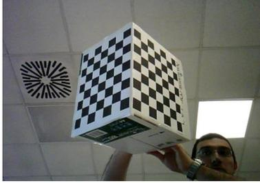
Figure 4.18: Snapshot of the calibration rig with Gumstix camera
