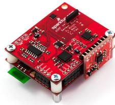
Figure 4.9: Inertial Measurement Unit
