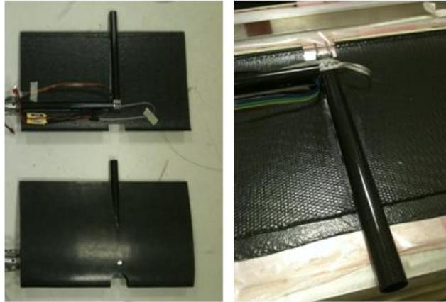
Figure 2.7: The spars and the landing gears inside the wings
