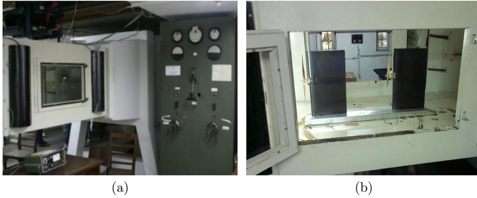
Figure 2.10: The wind tunnel (a) and the half prototype in the test room (b)
