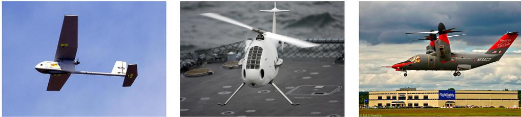
Figure 1.1: Fixed-Wing (Raven) [1], Rotary-Wing (Camcopter) [2] and VSTOL (BA609) [3] UAVs
