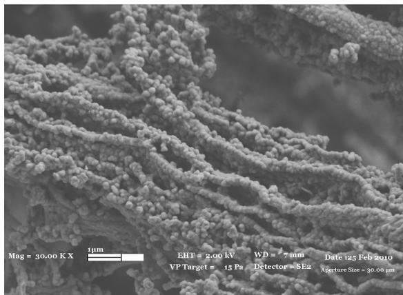
**Figure 3.** SEM image of PPy/graphene nanosheet-based nanocomposite
