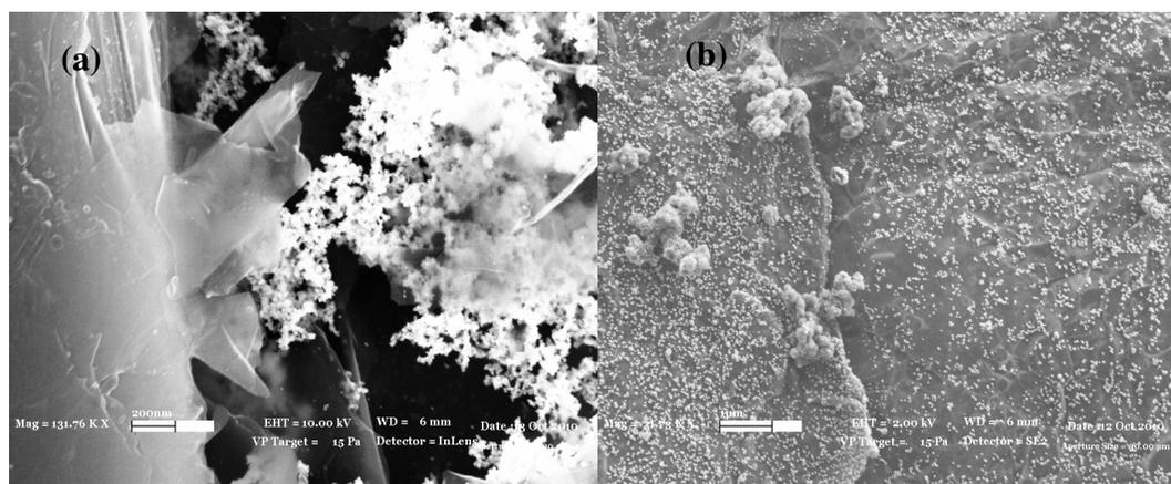
**Figure 5.** SEM images of (a) Pt/graphene nanosheets via inlens detector and (b) Pt/PPy/graphene nanosheets via secondary electron detector
