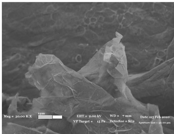
**Figure 2.** SEM image of graphene nanosheets after chemical reduction
