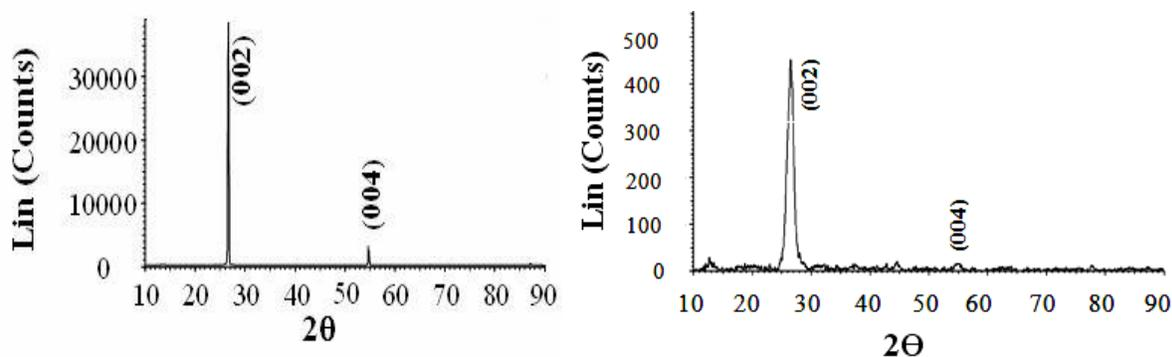
**Figure 2.** XRD patterns of (a) pristine graphite and (b) partially oxidized GO sheets
