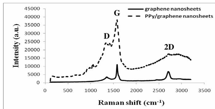
**Figure 4.** Raman spectra of graphene nanosheets and PPy/graphene nanosheets
