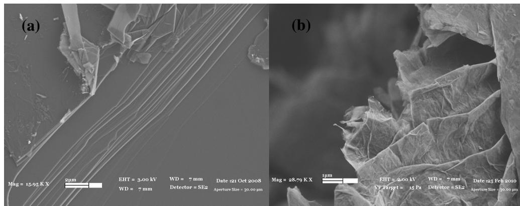
**Figure 1.** SEM images of (a) graphite flakes and (b) partially oxidized GO sheets
