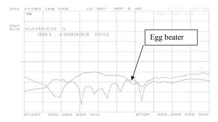
**Figure 4.** Measured SWR of the bent bowtie Maxon antenna at its input terminals of the hybrid coupler. The lower curve belongs to the commercial eggbeater antenna.
