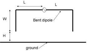
Figure 1. Bent dipole antenna over a ground plane
