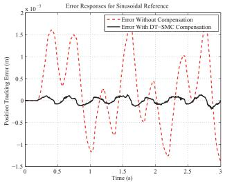
Fig. 8. Compensated and uncompensated tracking errors
