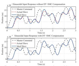
Fig. 7. Environment contact motion with sinusoidal input
