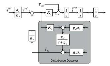
Fig. 1. Structure of the Disturbance Observer
