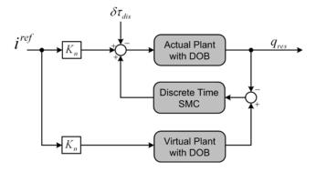
Fig. 5. Model following controller structure
