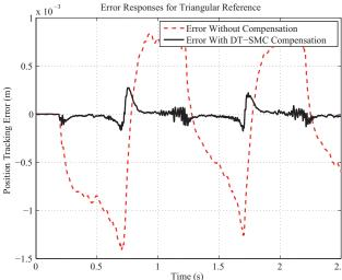
Fig. 10. Compensated and uncompensated tracking errors
