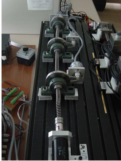
Figure 4.1: Lumped inertial system
