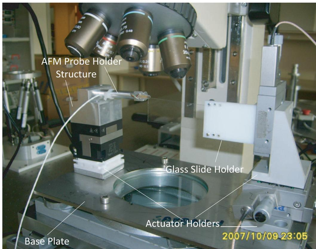
Figure 3.2: Custom built parts in the slave mechanism
