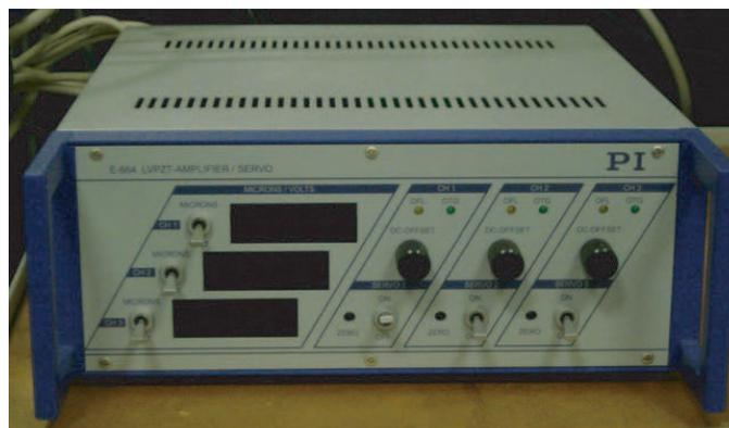
Figure 3.5: E664 NanoCube Piezo Controller
