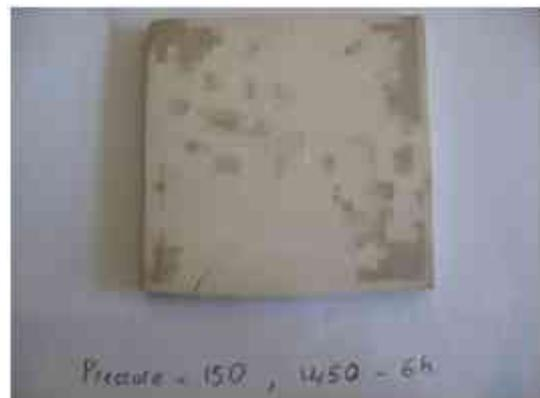
Fig 18 Substrate (layer 2) produced using compression pressure of :150Bar, Sintered at 1450C for 6h
