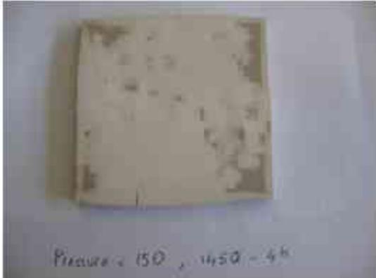
Fig 19 Substrate (layer 2) produced using compression pressure of :150Bar, Sintered at 1450C for 4h
