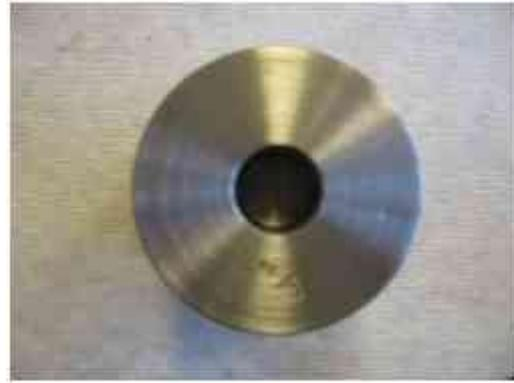
Fig 42 Last die used for pellet fabrication
