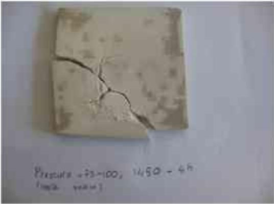
Fig 23 Substrate (layer2) produced using compression pressure of  $\approx 90$ Bar, Sintered at 1400C for 4h
