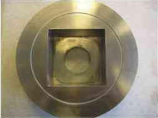
Fig 40 Last die (female part) for substrate fabrication
