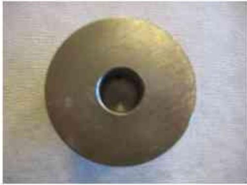
Fig 41 One of the previous dies manufactured for pellet fabrication
