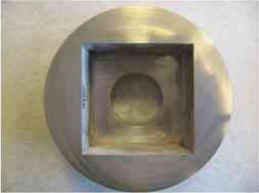
Fig 39 One of the previous dies (female part) manufactured for substrate fabrication
