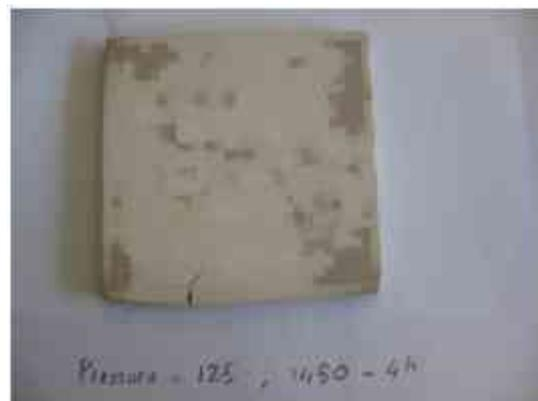
Fig 22 Substrate (layer2) produced using compression pressure of :125Bar, Sintered at 1450C for 4h
