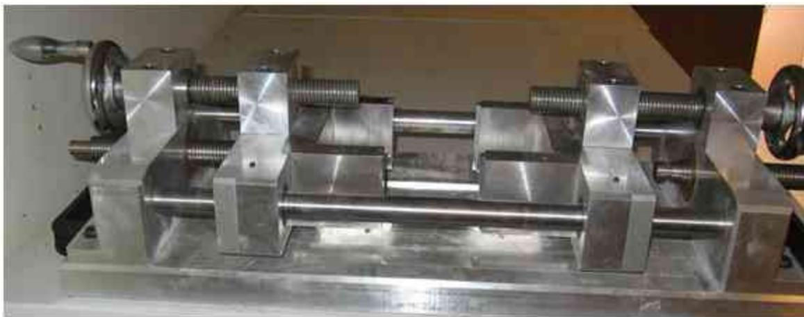
Fig 43 A different version of the die which can be adjusted according to desired substrate size
