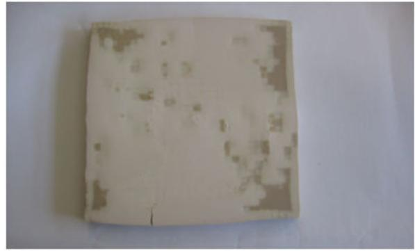
Fig 16 Substrate (layer 2) after sintering
