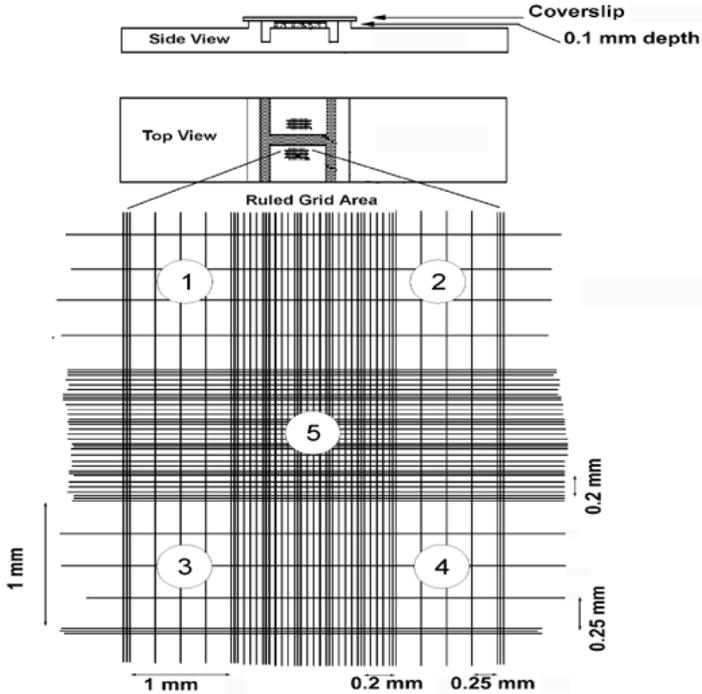
Fig. F.2. Schematic representation of a counting chamber on a hemacytometer. The area is divided into nine equal squares, five of which as depicted above are employed for counting.
